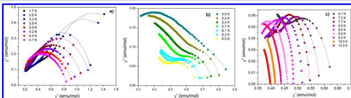
**Figure 7.** Argand plots and Debye fittings of the ac susceptibility of LYH:0.04Dy in the temperature range 1.7–10.5 K.  $H_{AC} = 5$  G;  $H_{DC} = 1000$  G.
