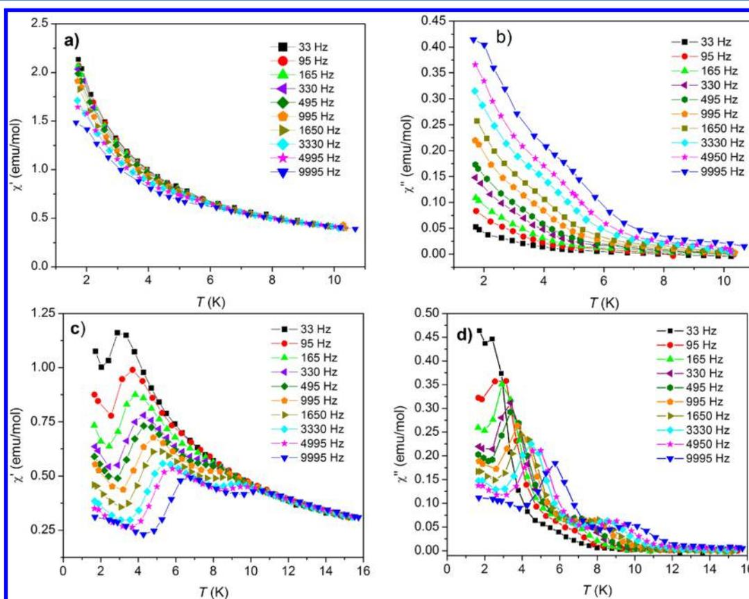
Figure 4. Temperature dependence of the real,  $\chi'$ , and imaginary,  $\chi''$ , components of the ac susceptibility for LYH:0.04Dy under different static fields,  $B = 0$  G (a and b) and  $B = 1000$  G (c and d), measured at different ac frequencies.
