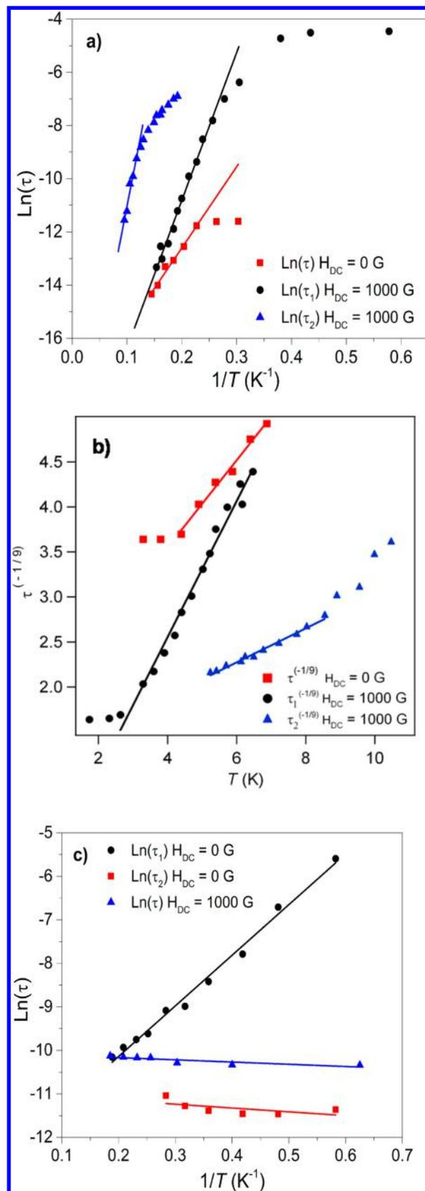
**Figure 9.** Thermal dependence of the relaxation time measured using ac fields  $H_{AC} = 5$  Oe and static magnetic fields indicated: (a) LYH:0.04Dy at  $H_{DC} = 0$  Oe (red) and  $H_{DC} = 1000$  G (process 2, blue triangles; process 1, black circles). Orbach process assumed (logarithm of the relaxation times versus inverse temperature). (b) LYH:0.04Dy
