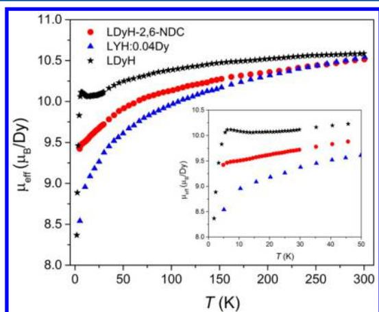
**Figure 2.** Effective magnetic moment of the dysprosium compounds in the temperature range 5–300 K obtained under a magnetic field of 100 G.
