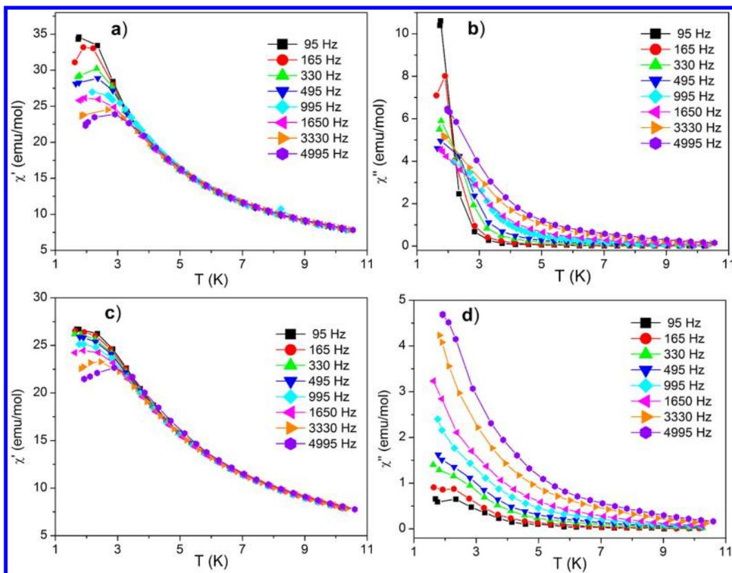
**Figure 5.** Temperature dependence of the real,  $\chi'$ , and imaginary,  $\chi''$ , components of the ac susceptibility for LDyH-2,6-NDC under different static fields:  $B = 0$  G (a and b) and  $B = 1000$  G (c and d), collected at different ac frequencies.
