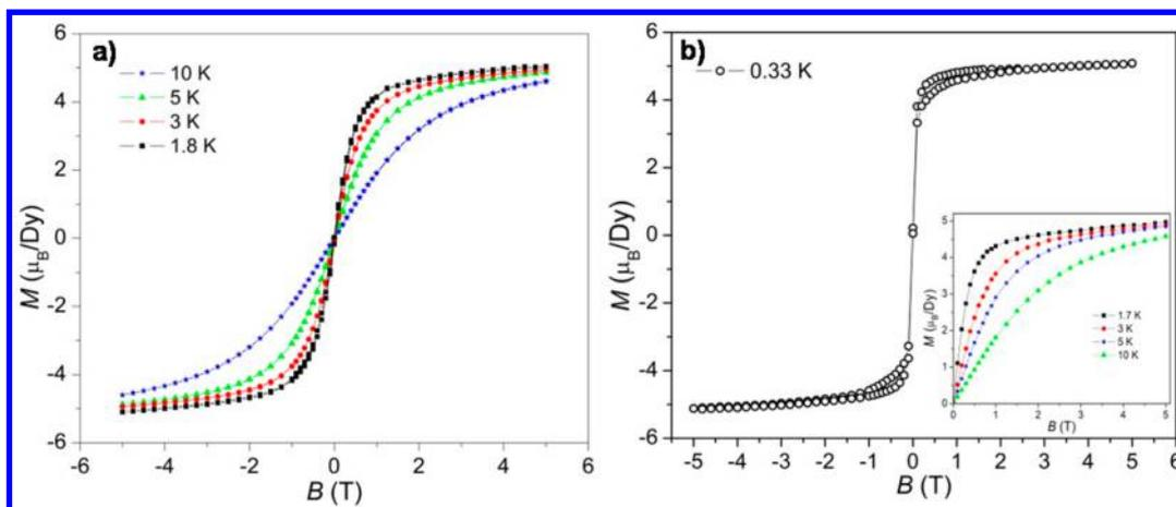
Figure 3. Field dependence of the magnetization at several temperatures for (a) LDyH-2,6-NDC and (b) LYH:0.04Dy compounds.
