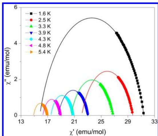
**Figure 8.** Argand plots and Debye fittings at different indicated temperatures in the range 1.6–5.4 K for LDyH-2,6-NDC.  $H_{AC} = 5$  G;  $H_{DC} = 1000$  G.
