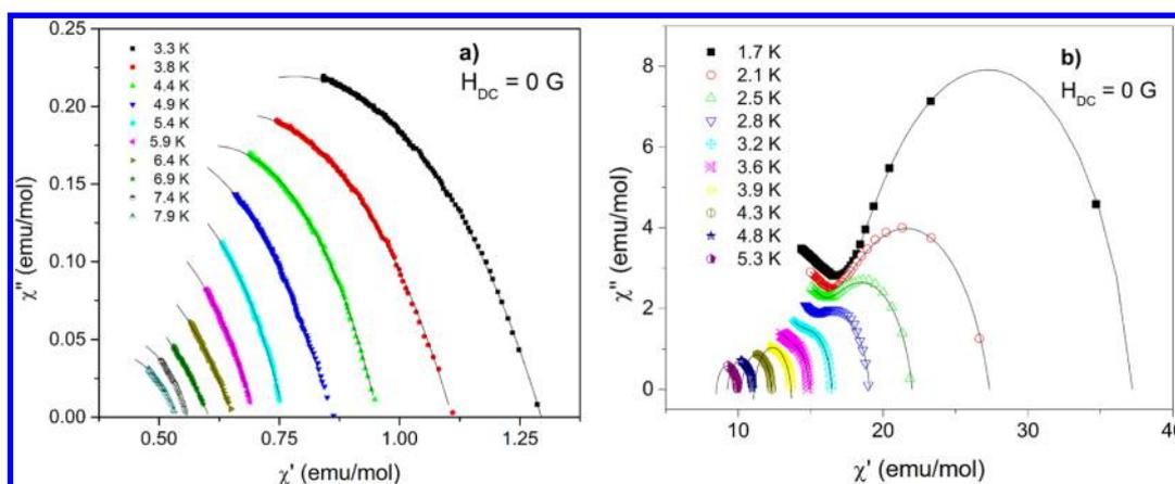
**Figure 6.** Argand diagrams and Debye fittings of the ac susceptibility for (a) LYH:0.04Dy and (b) LDyH-2,6-NDC at different temperatures indicated.  $H_{AC} = 5$  G;  $H_{DC} = 0$  G.
