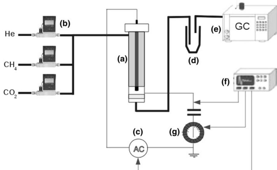
**Fig. 1** Experimental set-up: (a) DBD chamber, (b) mass flow controllers, (c) power supply, (d) trap, (e) gas chromatographer, (f) oscilloscope, (g) Rogowsky coil
