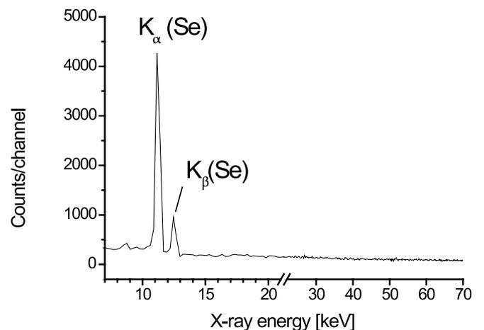
**Fig. 4.** X-ray spectrum of a radionuclidically pure  $^{76}\text{Br}$  sample taken with a Si(Li) detector.
