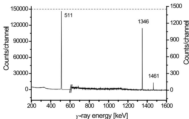
Fig. 2.  $\gamma$ -ray spectrum of a radionuclidically pure  $^{64}\text{Cu}$  sample taken with a HPGe detector.
