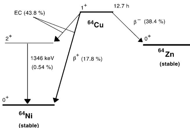
**Fig. 3.** Decay scheme of  $^{64}\text{Cu}$  with intensities of emitted radiations as determined in this work.
