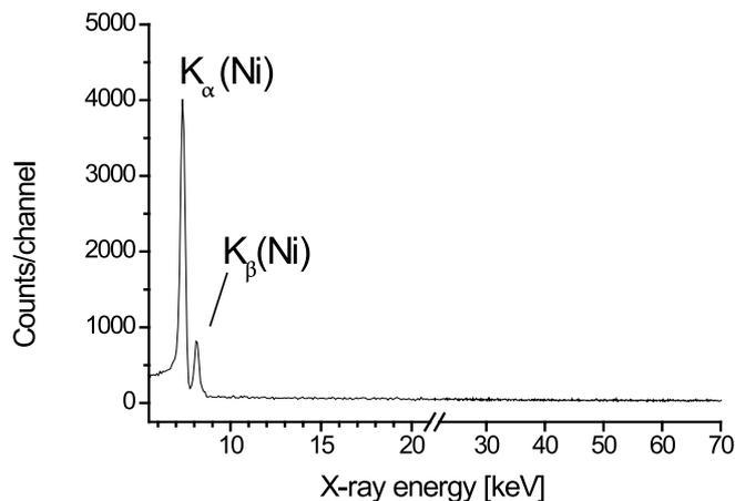
Fig. 1. X-ray spectrum of a radionuclidically pure  $^{64}\text{Cu}$  sample taken with a Si(Li) detector.
