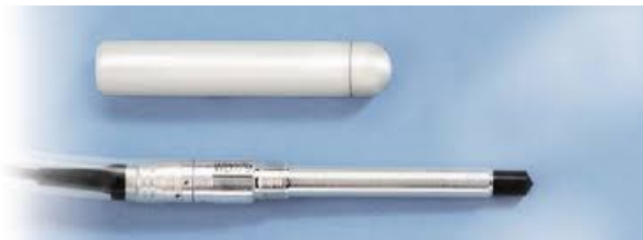
Figure 3.6: Photo of the ionization chamber used to measure the dose rate. Taken from [35].
