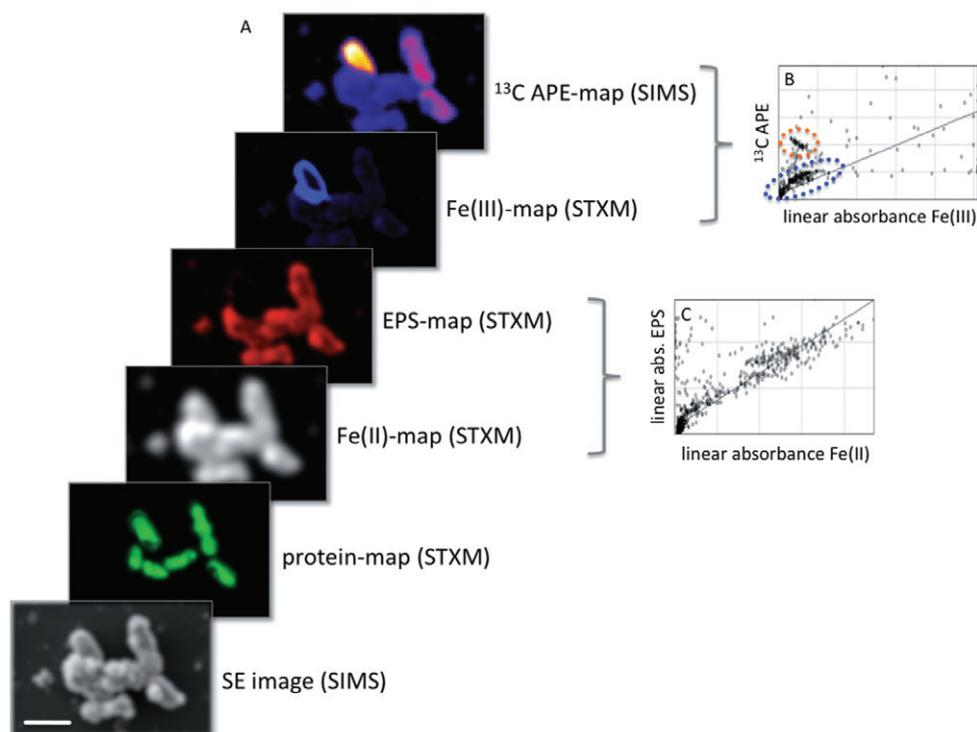
**Fig. 3.** A. Idealized schematic (no real data) of the correlative analysis of chemical species maps derived from SIMS and STXM. Atom per cent enrichment maps derived from SIMS analysis of stable isotope-labelled samples can be correlated to quantitative, linear absorbance maps of chemical or redox species derived from STXM analysis. Scale bar 1  $\mu\text{m}$ .
