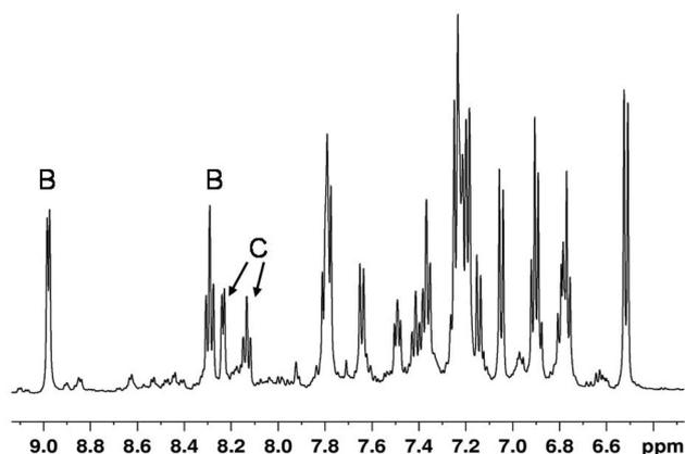
Fig. 6 Aromatic region of the  $^1\text{H}$  NMR spectra of  $[\text{GaL}^{\text{py},\text{NH}}]^+$  in  $\text{D}_2\text{O}$  showing the presence of two major isomers **B** and **C** in a 1:0.7 ratio. Minor peaks are from isomer **A**.
