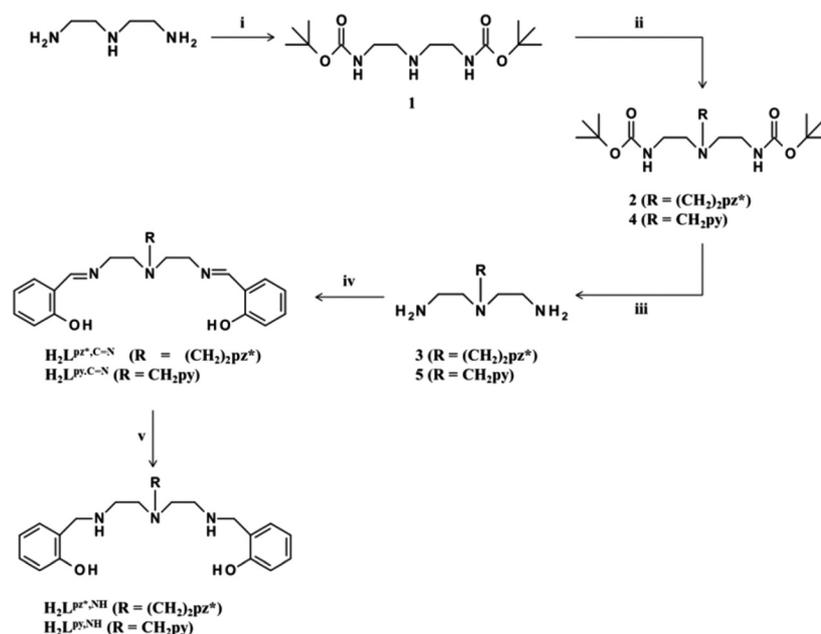
**Scheme 1** Synthesis of the ligands. (i)  $\text{O}(\text{BOC})_2$ , THF, r.t., o.n.; (ii)  $\text{BrCH}_2\text{CH}_2(3,5\text{-Me}_2\text{pz})$  or  $2\text{-BrCH}_2\text{py}$ ,  $\text{K}_2\text{CO}_3$ , KI, THF, reflux, 24 h; (iii) HCl/MeOH, r.t., 2 h; (iv) salicylaldehyde, MeOH, reflux, 4 h; (v)  $\text{NaBH}_4$ , MeOH, r.t., o.n.
