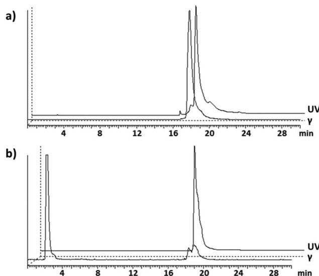
Fig. 7 HPLC chromatograms of: (a)  $[\text{GaL}^{\text{py},\text{NH}}](\text{ClO}_4)$  (UV detection) and the reaction mixture of the radiolabeling of  $\text{H}_2\text{L}^{\text{py},\text{NH}}$  with  $^{67}\text{GaCl}_3$  ( $\gamma$  detection); (b)  $[\text{GaL}^{\text{pz}^*,\text{NH}}](\text{ClO}_4)$  (UV detection) and the reaction mixture of the radiolabeling of  $\text{H}_2\text{L}^{\text{pz}^*,\text{NH}}$  with  $^{67}\text{GaCl}_3$  ( $\gamma$  detection).
