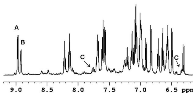
Fig. 4 Aromatic region of the  $^1\text{H}$  spectrum of  $[\text{GaL}^{\text{py},\text{NH}}]^+$  in  $\text{CD}_3\text{CN}$  showing the presence of two major isomers A and B in a 1:0.6 ratio. Some of the peaks of the minor species C are also identified.
