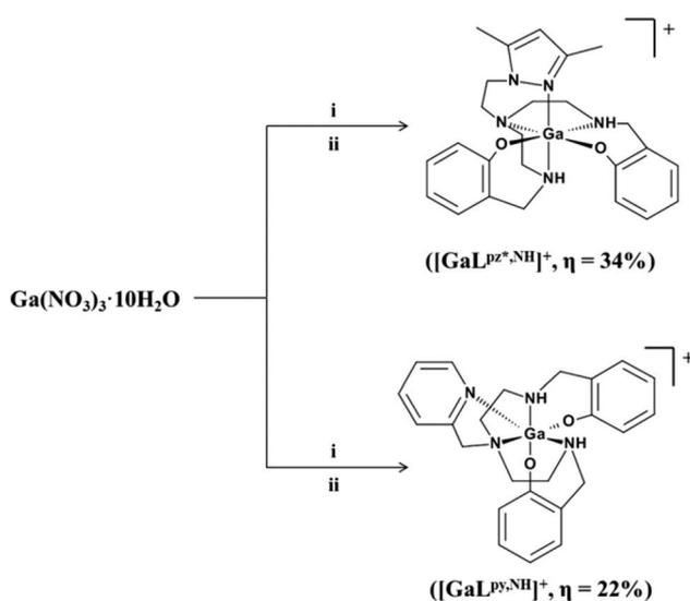
**Scheme 2** Synthesis of the gallium complexes. (i)  $\text{H}_2\text{L}^{\text{pz}^*,\text{NH}}$  or  $\text{H}_2\text{L}^{\text{py},\text{NH}}$ ,  $\text{NaCH}_3\text{COO}$ ,  $\text{MeOH}$ , r.t., o.n.; (ii)  $\text{NaClO}_4$ .
