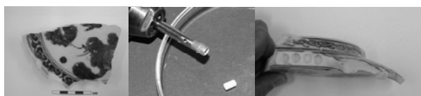
Figure 1. Drilling of core sample: d.= 3 mm, l.= 5 mm.
