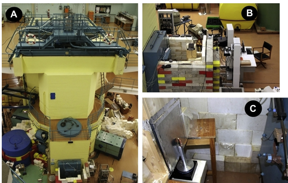
Fig. 3. Images of the neutron tomography (NT) setup of the Portuguese Research Reactor (RPI): A. general view of the RPI, with the NT setup (middle, bottom); B. NT setup; C. detail of the neutron window and the rotary table with the MNA tile sample.
