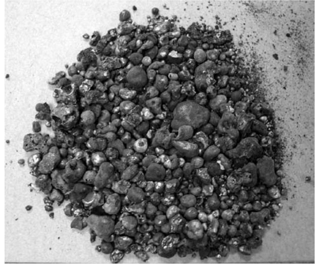
Fig. 4: Metal prills after crushing the slag. Scale in mm.
