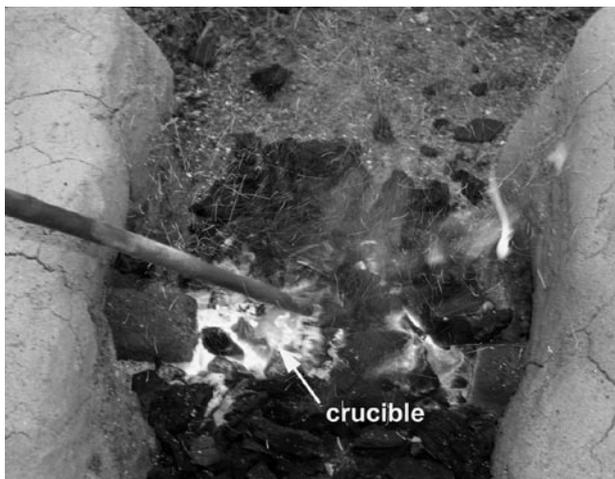
Fig. 3: Charge. The arrow points to a handful of crushed ore on top of the burning charcoal.
