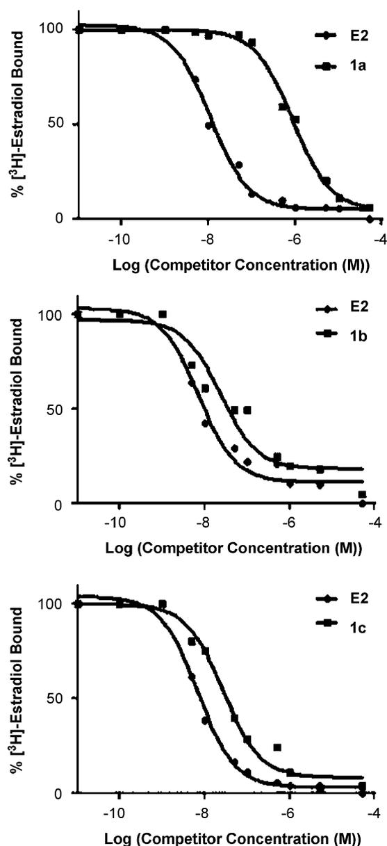
Fig. 2. Comparison of the relative ER-binding affinity of compounds **1a**, **1b** and **1c** with that of estradiol ( $\text{E}_2$ ). The relative binding affinity of each competing compound was determined by measuring its inhibition of the binding of [ $^3\text{H}$ ] $\text{E}_2$  to the recombinant human ER $\alpha$ . The data for nine concentrations ( $1\text{--}5 \times 10^4 \text{ nM}$ ) was taken. Each point represents the mean of duplicate measurements.
