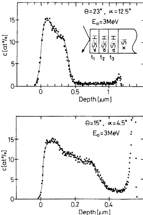
Fig. 7. H depth-profile in a-Si:H multilayer on Si at different analysing conditions. The  $t_1$ ,  $t_2$ ,  $t_3$  deposition temperatures are  $150$ ,  $250$  and  $350^\circ\text{C}$  respectively. Note the improved depth resolution at  $\alpha = 4.5^\circ$ . At high depth, the peak arises from noise.
