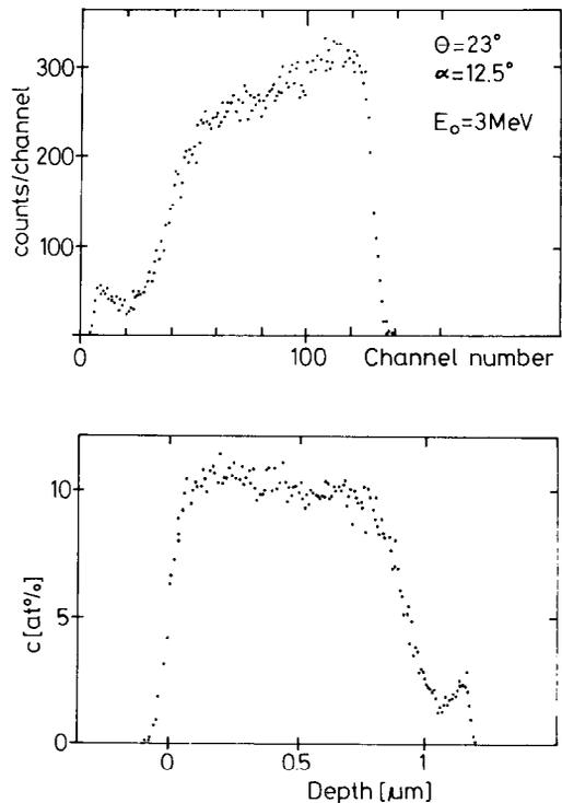
Fig. 6. The ERD spectrum and the conversion to H depth-profile in a-Si:H layer deposited onto Si. The layer thickness and deposition temperature was  $0.9 \mu\text{m}$  and  $350^\circ\text{C}$  respectively. At low energies, the peak comes from noise.
