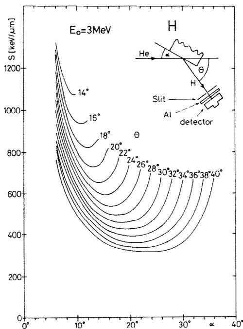
Fig. 4. Energy loss factor in Si substrate for He recoiled protons as a function of  $\alpha$  and  $\theta$ .
