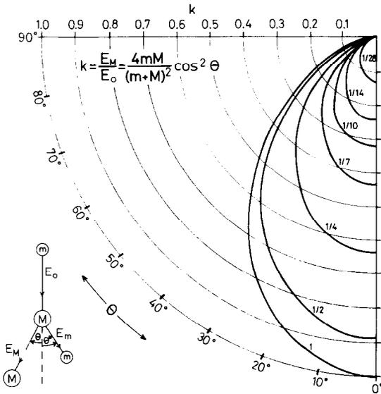
Fig. 1. Kinematic factor for the energy of recoiled particles. The plotting parameters are  $M/m$  ratios.
