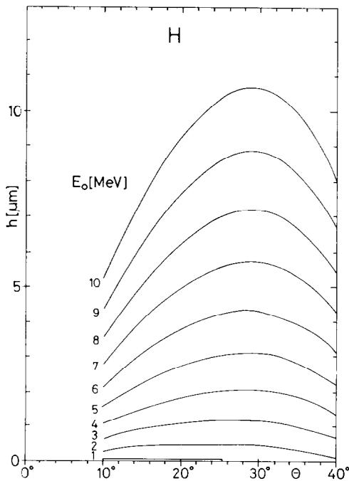
Fig. 5. The maximum analysis depth for H in Si vs.  $\theta$  at different incident energies.
