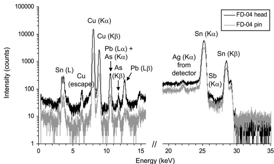
Fig. 4. EDXRF spectra of the nail FD-04 performed over the convex side of the head and over the pin (different intensities can be attributed to differences in the analysed areas that are due to the different sizes of the pieces).
