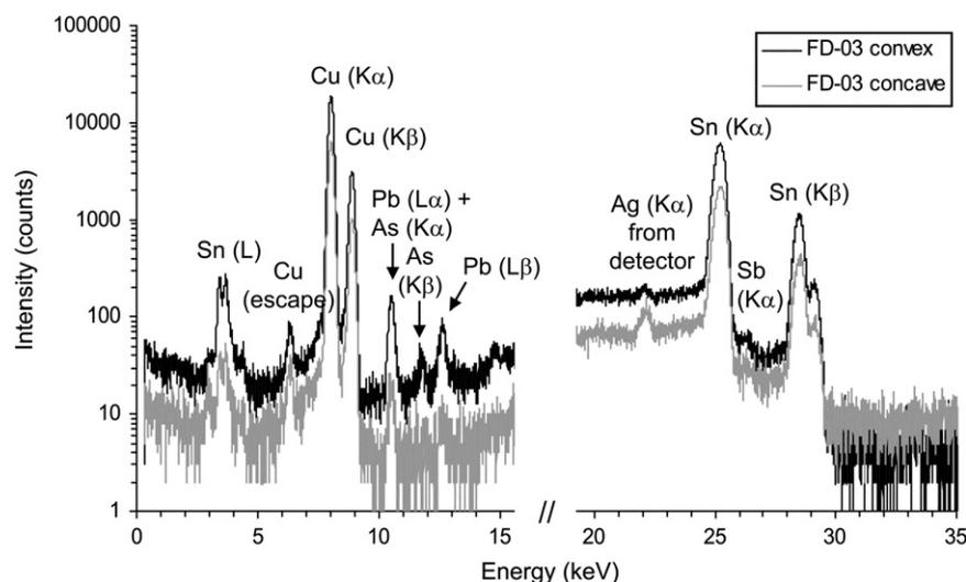
**Fig. 5.** EDXRF spectra of the head of the nail FD-03 performed over the convex and concave sides (different intensities are due to geometrical factors caused by the different surface shapes).
