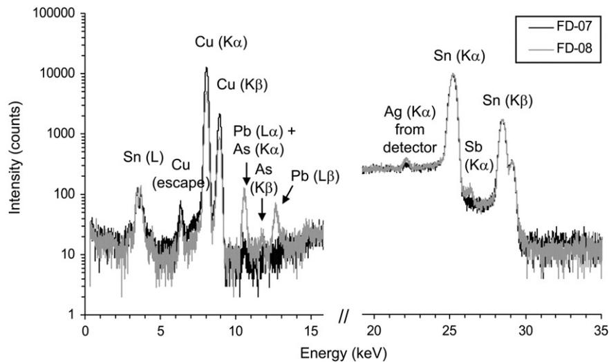
Fig. 3. EDXRF spectra of dagger (FD-07) and sickle (FD-08).
