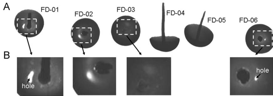
**Fig. 6.** X-ray radiograph of the six nails from Figueiredo das Donas. (A) General view and (B) detailed images of the regions around the junction of the pin and head of FD-01, FD-02, FD-03 and FD-06 nails.
