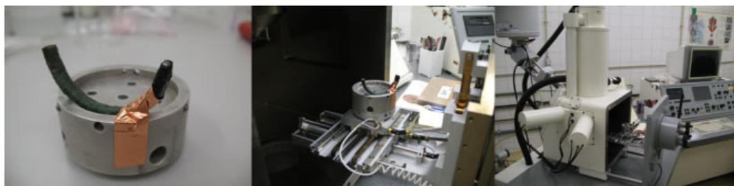
**Figure 2.** On the left is an image of the preparation of a bronze bracelet fragment from Medronhal cave (Central Portugal) for SEM-EDS analysis, with the enveloping of corroded surfaces with copper and carbon tape near the prepared and cleaned area, leaving the latest uncovered for analysis (the analysed area is the top right surface). The centre and right images show the placing of the artefact in the SEM-EDS chamber.
