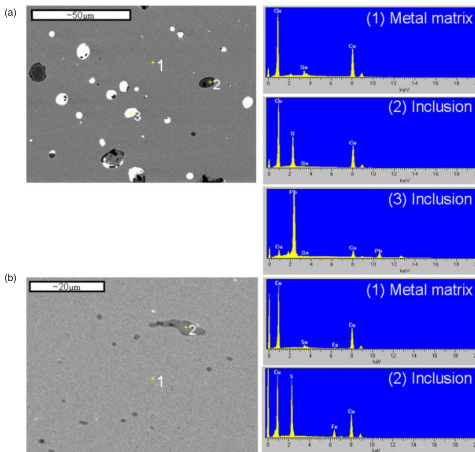
**Figure 9.** (a) SEM/BSE image of a bronze bar fragment from Fraga dos Corvos shelter (North Portugal) with inclusions that follow the dendritic solidification path, and spot EDS analysis of (1) metal matrix, (2) inclusion of Cu-S and (3) inclusion of Pb (bronze with ~2 wt% Pb by micro-EDXRF). (b) SEM/BSE image of a bronze rod from Palhais (South Portugal) with inclusions, and spot EDS analysis of (1) metal matrix, (2) inclusion of Cu-S-Fe.
