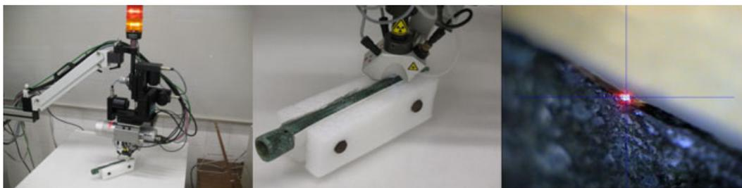
**Figure 1.** The ArtTAX Pro spectrometer during the analysis of a bronze spearhead from Penela (Central Portugal). On the right is an image obtained by the CCD camera during the selection of the measuring location. Here, in conjunction with a laser spot and crosshairs on the video display the reproducible settings of the measuring distance and location of the measured spot are assured (principle of optical triangulation, see also Ref. [13]).
