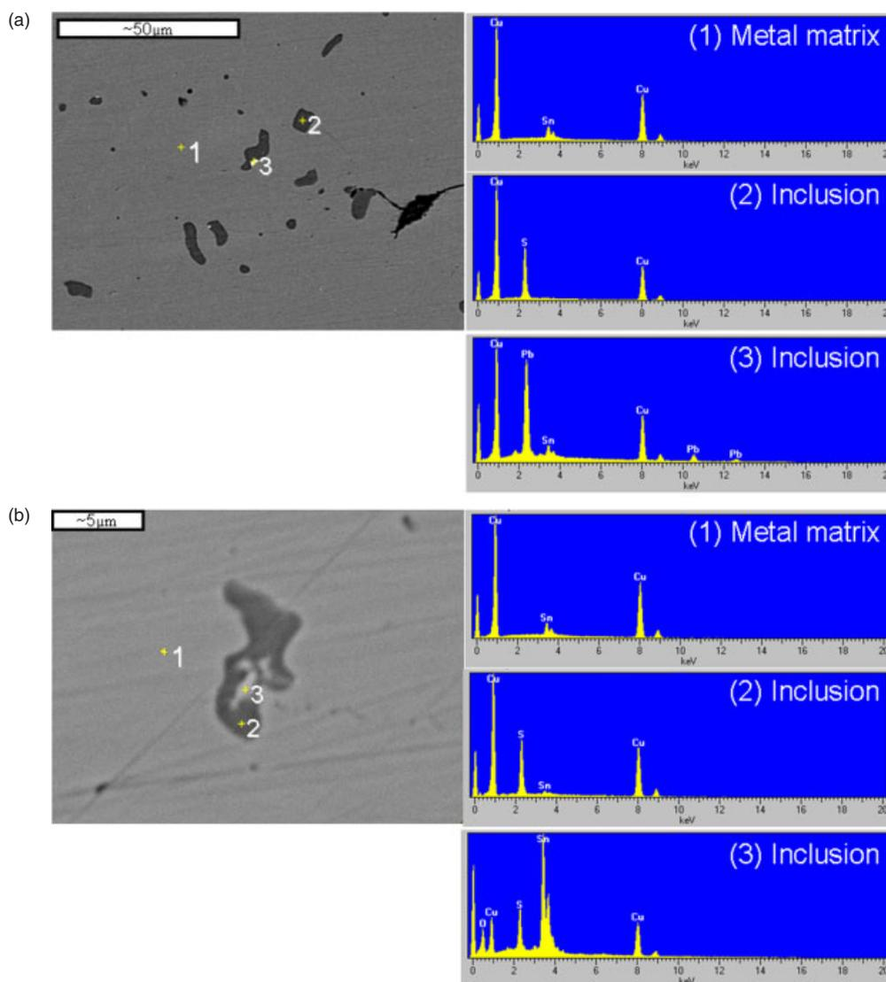
**Figure 6.** (A) SEM/BSE image of a bronze bracelet fragment from Medronhal cave (Central Portugal) with inclusions, and spot EDS analysis of (1) metal matrix, (2) inclusion of Cu–S and (3) inclusion of Pb. (B) SEM/BSE image of a bronze ring from the same site with an inclusion and spot EDS analysis of (1) metal matrix, (2) inclusion of Cu–S and (3) inclusion of Sn–O (due to the small size of some inclusions, the EDS spectrum also contains additional information from the surrounding area).
