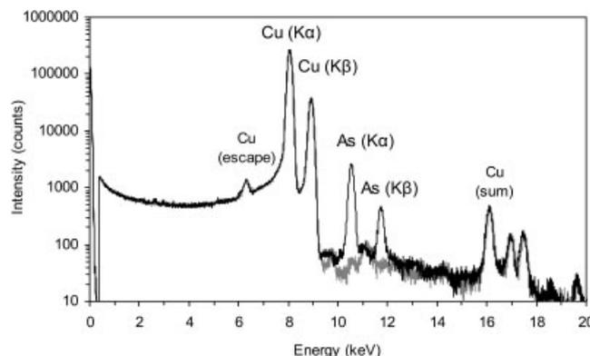
**Figure 3.** Micro-EDXRF spectra of a relatively pure copper fragment from Escoural archaeological site (South Portugal) (in grey), and a copper rivet with  $\sim 2$  wt% As from Folgão (South Portugal) (in black).
