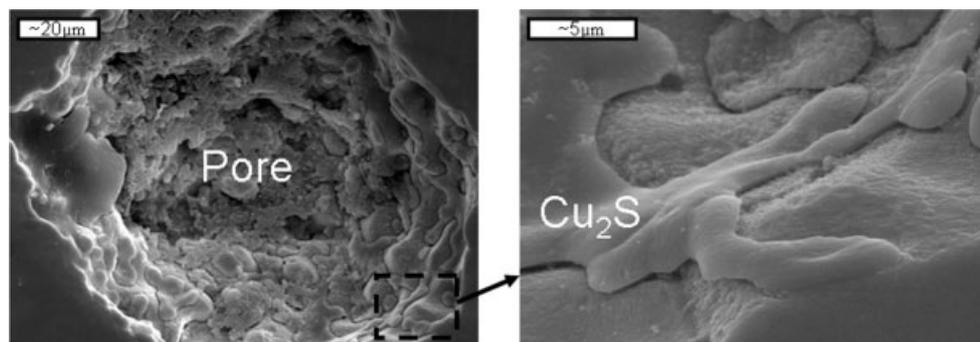
**Figure 7.** SEM/SE image of a pore in a bronze bar fragment from Santa Luzia archaeological site (Central Portugal) with the walls covered by copper sulphides as a result of microsegregation.
