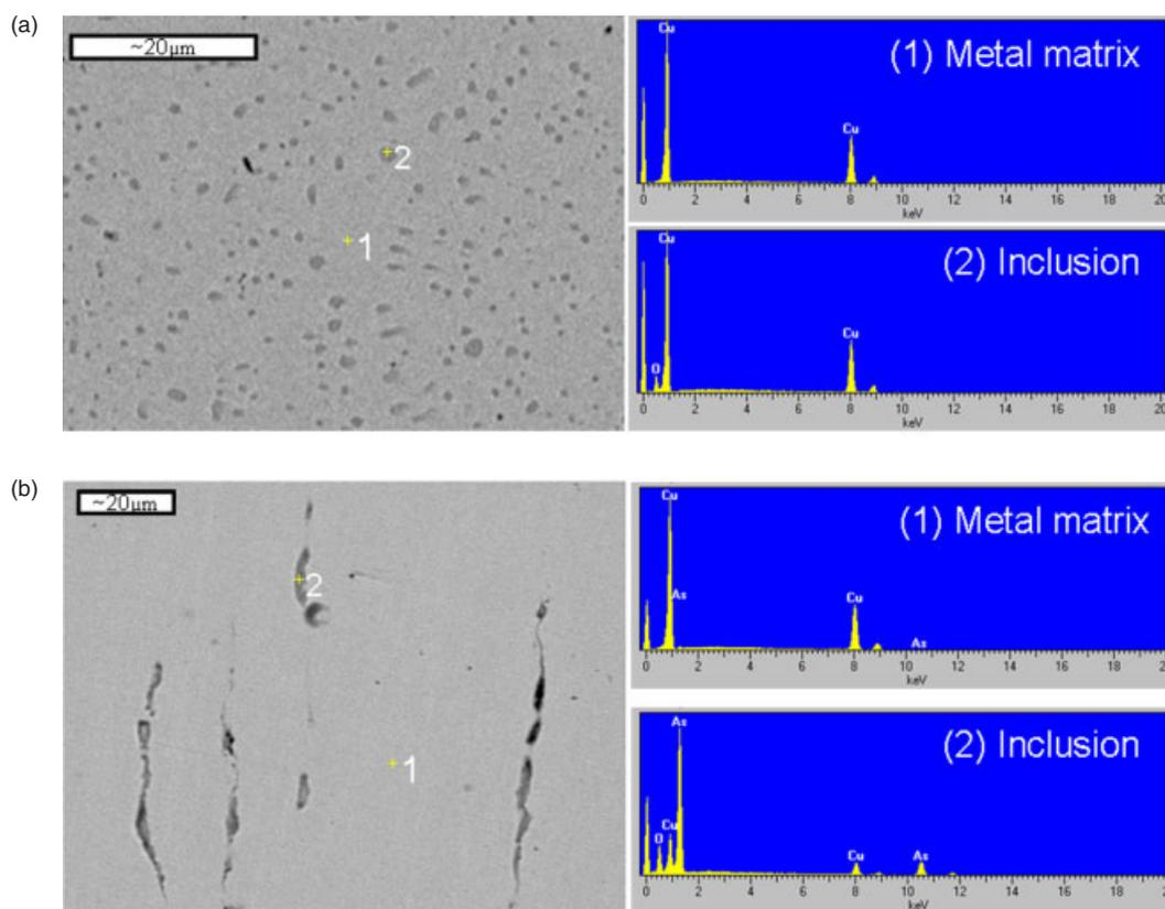
**Figure 4.** (a) SEM/BSE image of a relatively pure copper fragment from Escoural archaeological site (South Portugal) with inclusions (darker grey) and EDS analysis of (1) the metal matrix and (2) inclusion of Cu-O. (b) SEM/BSE image of a copper rivet with  $\sim 2$  wt% As (micro-EDXRF) from Folgão (South Portugal) with elongated (deformed) inclusions due to significant mechanical work on the artefact, and EDS analysis of (1) the metal matrix and (2) inclusion with Cu-As-O.
