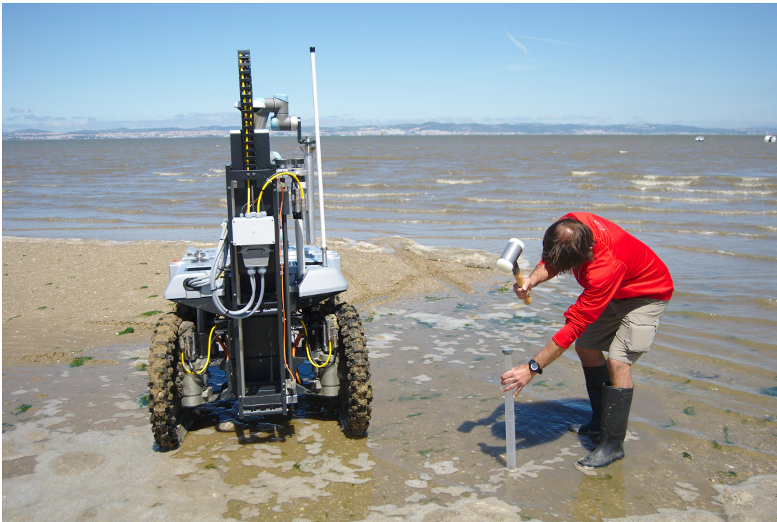
Figure 2. The ground vehicle drilling the terrain side-by-side a human expert handling a conventional manual tool. The human expert hammers an acrylic hollow cylinder until a desired depth is reached. Then, the cylinder must be gently pulled in order to ensure that the sediments do not fall. All of this process is time consuming and physically demanding. Conversely, the robot drills effortlessly and stores up to nine samples before it needs to return to the base.
