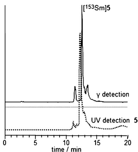
**Figure 3.** HPLC chromatograms of the nonradioactive complex **5** (UV detection at 254 nm; dotted trace; retention time ( $t_R$ ) = 12.4 min) and the radioactive analogue [ $^{153}\text{Sm}$ ]**5** ( $\gamma$  detection;  $t_R$  = 12.5 min). Under the same conditions, the free  $^{153}\text{Sm}$  species has an  $t_R$  value of 2.5 min.
