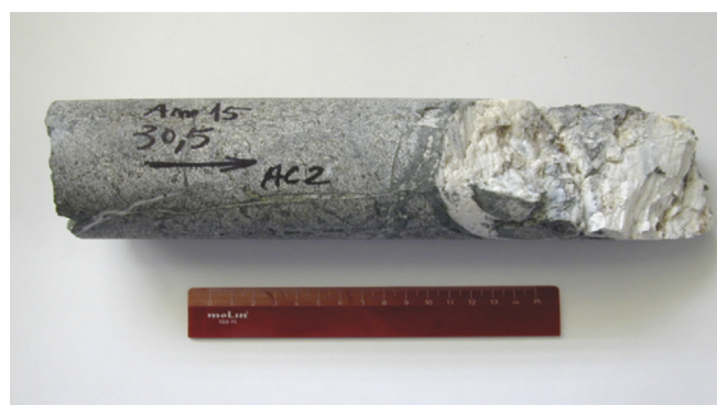
Fig. 4. Drillcore from the exploration borehole AC2 (CdV Spa). Serpentinized peridotite, showing strong serpentinization along the rock fractures.
