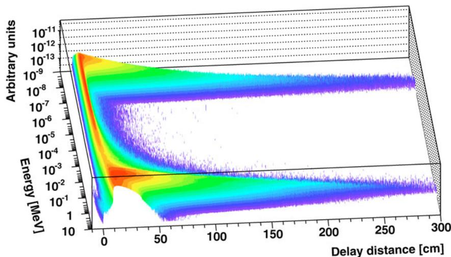
Fig. 2. Two-dimensional matrix of the tallied quantities in MCNPX, showing their dependence.
