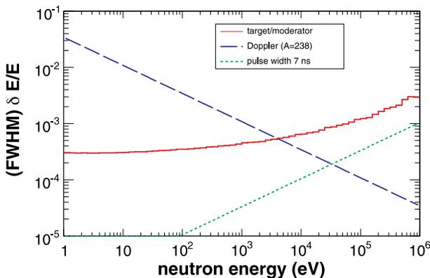
Fig. 8. Different contributions for the broadening of the resonances. The target/moderator curve represents the results obtained for the FWHM with MCNPX using a moderation depth of 5 cm.
