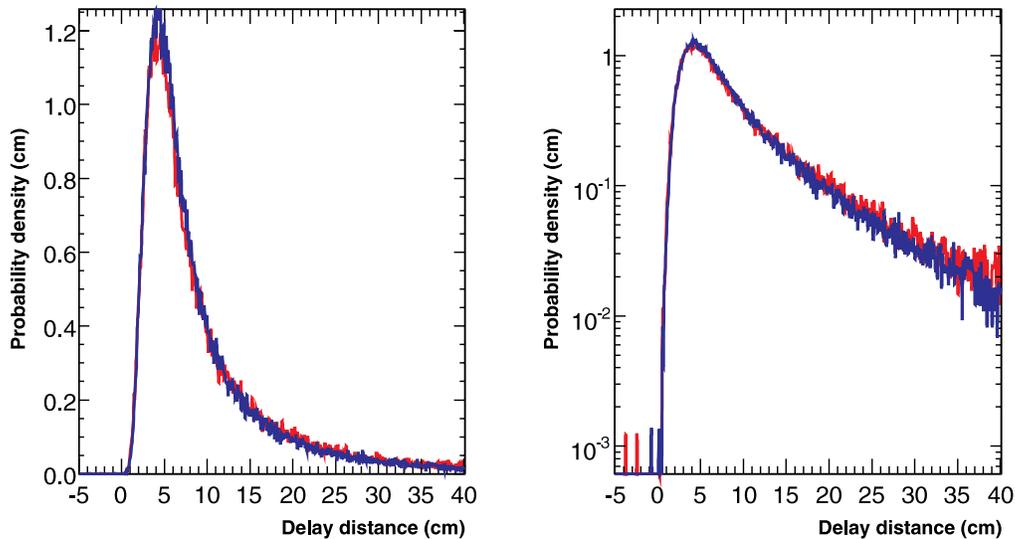
Fig. 7. Comparison of the equivalent distance between two different moderation depths for 8 keV (red for 5 cm and blue for 5.8 cm) (color online).
