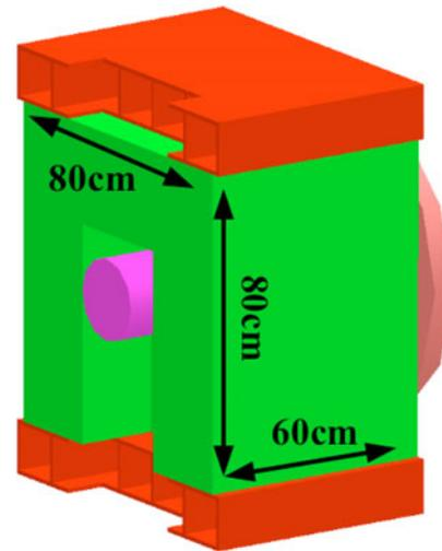
Fig. 1. Target system accompanied by the supporting structure and aluminum entrance window on the right. The proton beam impinges from the left side.
