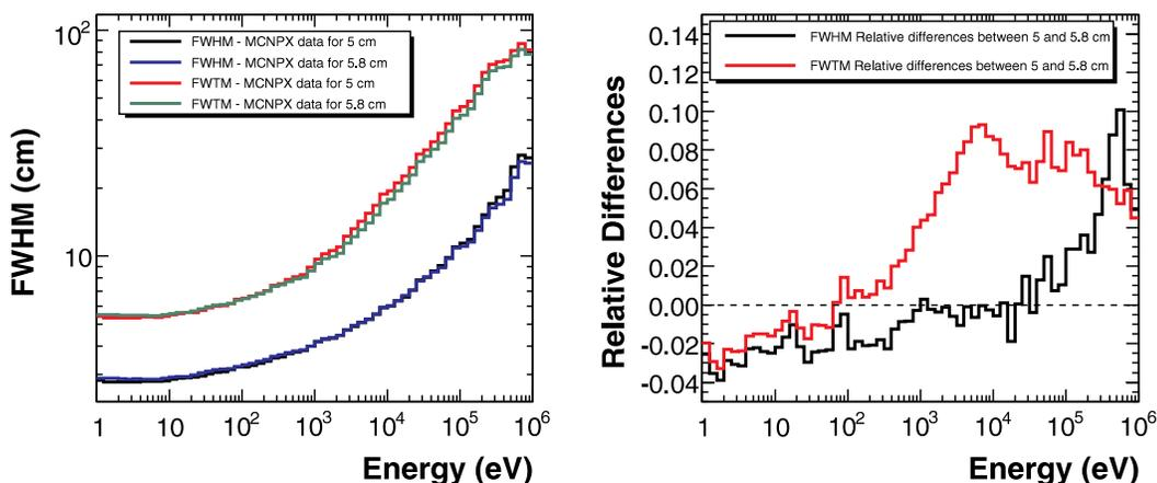
Fig. 6. The FWHM and the FWTM for 5 and 5.8 cm of moderation depth simulated with MCNPX.
