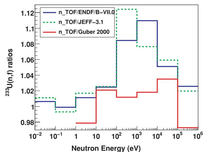
FIG. 10. (Color online) Ratio of the n\_TOF results with previous data and evaluations averaged over neutron energy decades. The present results indicate a deficiency of 10% in the evaluated data between 100 eV and 10 keV, a region of interest for advanced nuclear reactor technology. The comparison between n\_TOF and Guber's data in the last bin is performed up to the maximum energy of 700 keV.
