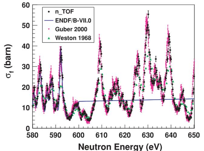
FIG. 8. (Color online) The  $^{233}\text{U}(n, f)$  cross section at the limit of the resolved resonance region in ENDF/B-VII.0. Well-resolved resonances are observed at n\_TOF above this limit, in agreement with recent results of Ref. [29]. Previous results of Ref. [31] are shown for comparison.
