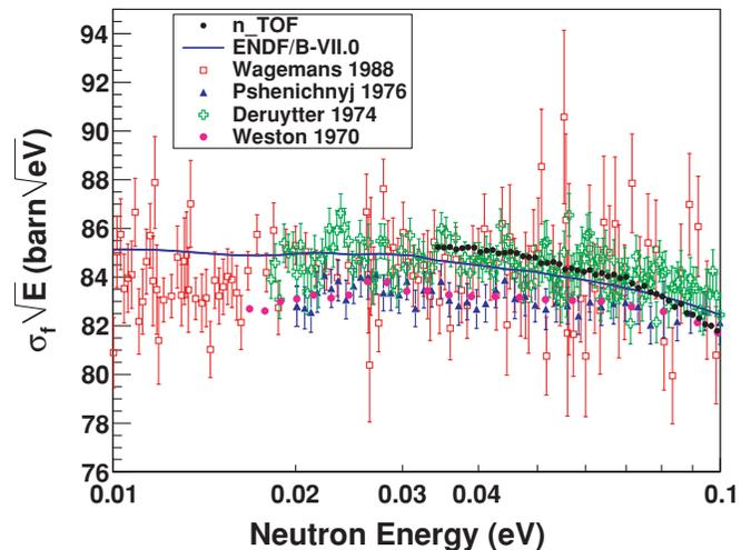
FIG. 5. (Color online) Velocity-weighted fission cross section from 10 meV to 0.1 eV. The n\_TOF results (black symbols) are compared with the ENDF/B-VII.0 evaluated data (blue curve), and with previous measurements. The data of Wagemans *et al.* [23], which extends down to 2 meV, and Deruytter *et al.* [25] are normalized to the thermal ENDF/B-VI cross section of 531.14 b. The statistical uncertainties of n\_TOF results are included and are as small as the symbols.
