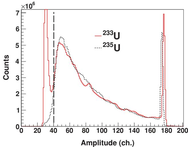
FIG. 1. (Color online) Pulse height spectra for the  $^{233}\text{U}$  sample and for the  $^{235}\text{U}$  reference sample. The threshold for discriminating fission fragments from  $\alpha$  background and electronic noise is indicated by the dotted line at channel 40. The peaks observed close to channel 180 are due to a saturation effect of the flash-ADC.
