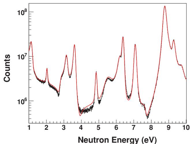
FIG. 2. (Color online) Measured  $^{235}\text{U}$  counting rate in the energy region from 1 to 10 eV (black line), compared to the ENDF/B-VII.0 evaluation (red line), normalized at the first  $^{235}\text{U}(n, f)$  resonance.
