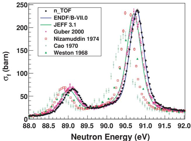
FIG. 7. (Color online) Resonances in the  $^{233}\text{U}(n, f)$  cross section measured at n\_TOF around 90 eV. Large discrepancies between previous data [30–32] and evaluations are evident. In this region, the n\_TOF results confirm the evaluated data from ENDF/B-VII.0, while better agreement is observed with JEFF 3.1 in other regions. n\_TOF data are given with statistical uncertainties.
