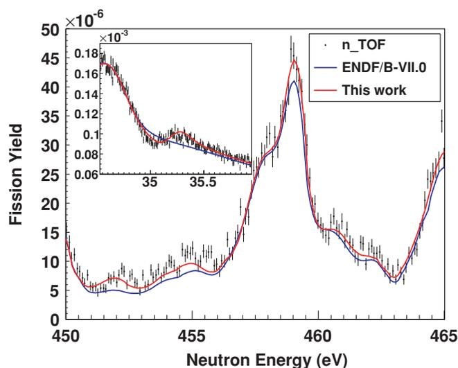
FIG. 11. (Color online) The measured and fitted n\_TOF data compared with a fit based on the resonance parameters of Ref. [39] in the energy range 450 to 465 eV. The inset shows an example of a new resonance found in the present data.
