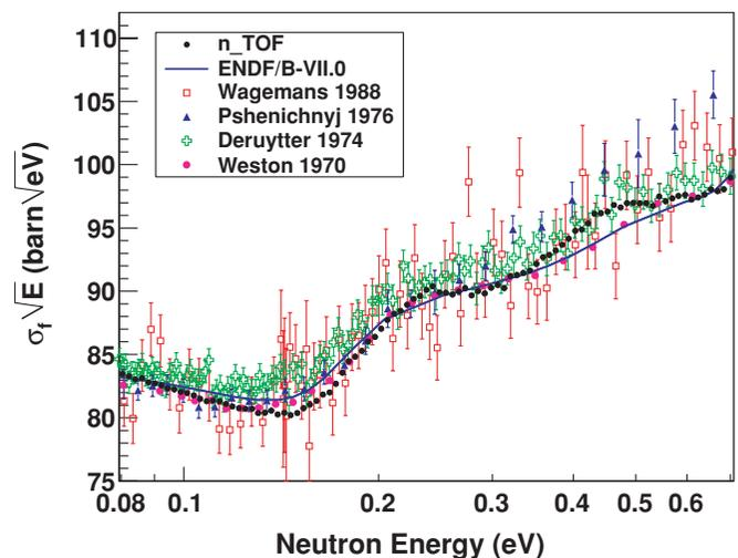
FIG. 6. (Color online) Velocity-weighted fission cross section from 0.1 to 0.8 eV. The n\_TOF results (black symbols) are compared with previous measurements and with the ENDF/B-VII.0 database (blue curve). Two resonances at 0.25 and 0.45 eV are clearly observed in the n\_TOF data. The statistical uncertainties of n\_TOF results are included and are as small as the symbols.
