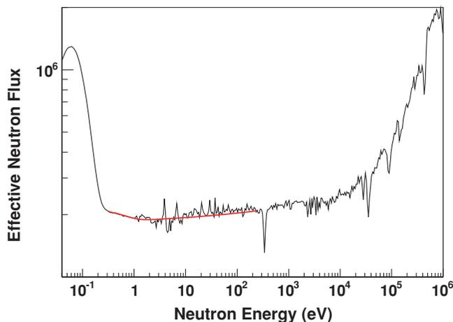
FIG. 3. (Color online) Isolethargic distribution of the effective neutron flux (i.e., the product between efficiency and neutron flux), expressed as  $dn/d \ln E$  per  $7 \times 10^{12}$  protons and measured with the FIC detector via the  $^{235}\text{U}(n, f)$  reaction (black histogram). The red line indicates the flux used in the present analysis between 0.16 and 245 eV, which was obtained as described in the text.
