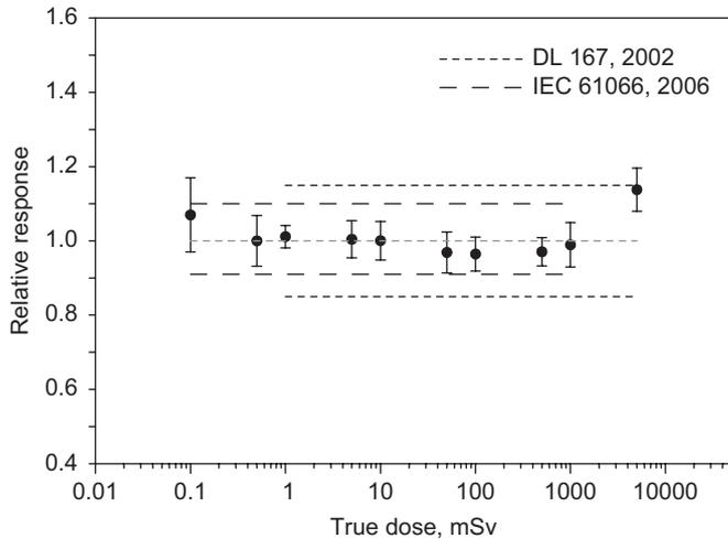
Fig. 3. Linearity curve for 0.1 mSv to 5 Sv dose range. Irradiations performed in the <sup>137</sup>Cs radiation beam.
