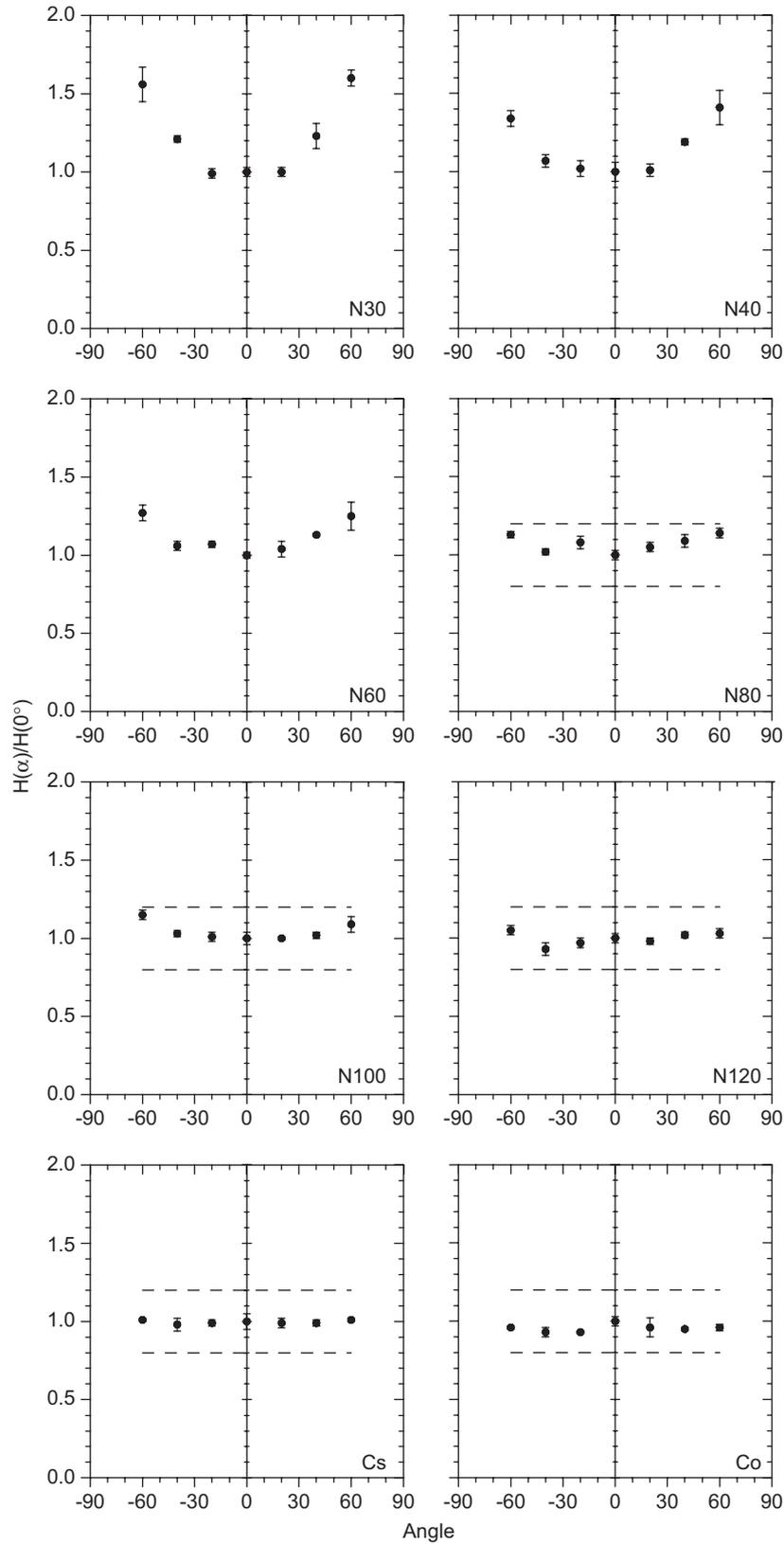
Fig. 5.  $H_p(10)$ : angular dependence for all irradiation beams studied.
