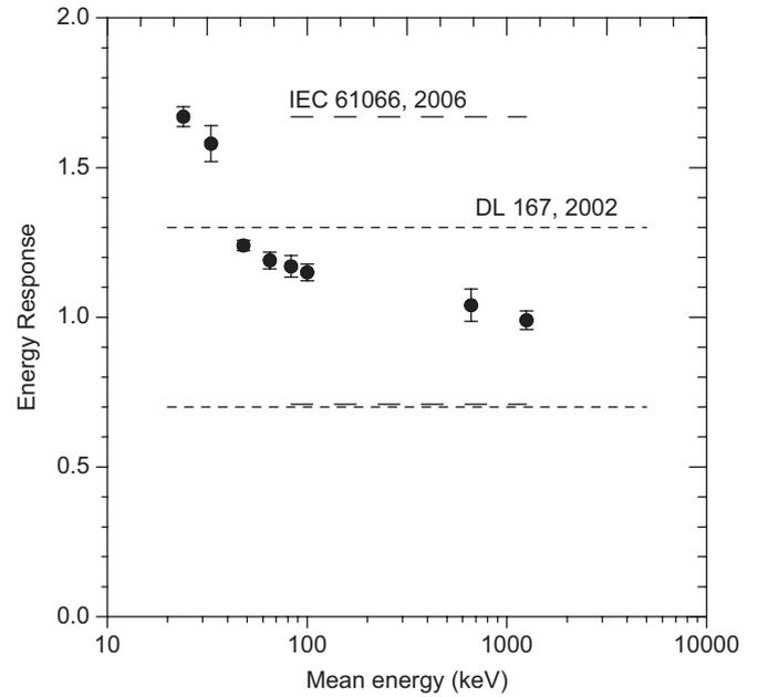
Fig. 4. Energy dependence for normal incidence normalized to <sup>137</sup>Cs.
