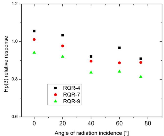
Fig. 5. Angular  $H_p(3)$  response of the new EYE-D<sup>TM</sup> dosimeter for RQR spectra (normalized to response to Cs-137 gamma rays, normal incidence).
