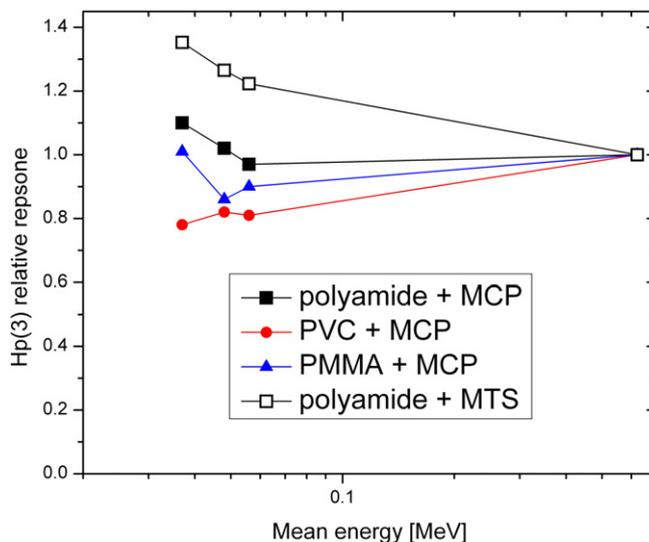
Fig. 2. The measured photon energy response of the tested dosemeter configurations.
