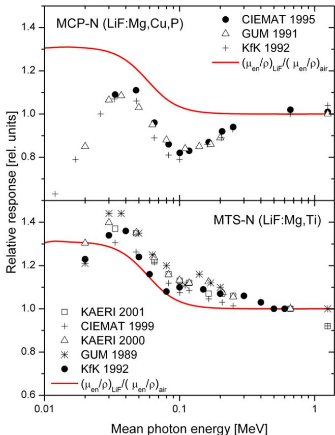
Fig. 1. Photon energy response of LiF:Mg,Cu, P (MCP-N) and LiF:Mg,Ti (MTS-N) as measured in several experiments. Solid lines indicate dependence of the mass energy absorption coefficient (after Olko, 2002).
