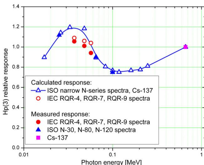
Fig. 4. Calculated (open symbols) and measured (full symbols)  $H_p(3)$  response of the new EYE-D<sup>TM</sup> dosimeters for RQR and ISO N X-ray spectra.
