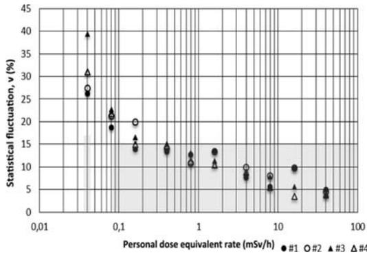
Figure 5. Results on the dose rate statistical fluctuations.
