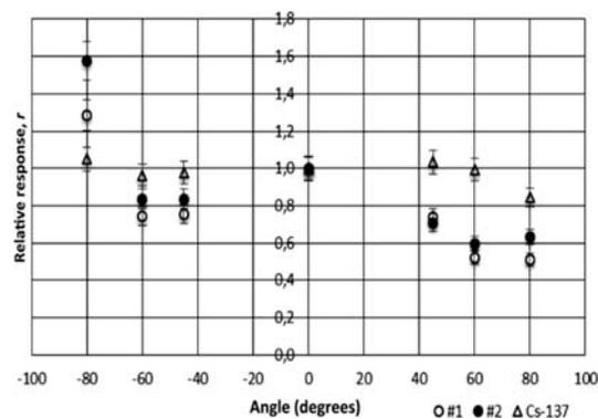
Figure 4. Angle dependence of the personal Dosimeters 1 and 2, relative response at 5 mSv/h for N-100. For Cs-137 radiation quality, the relative response of Dosimeter 1 is also presented.
