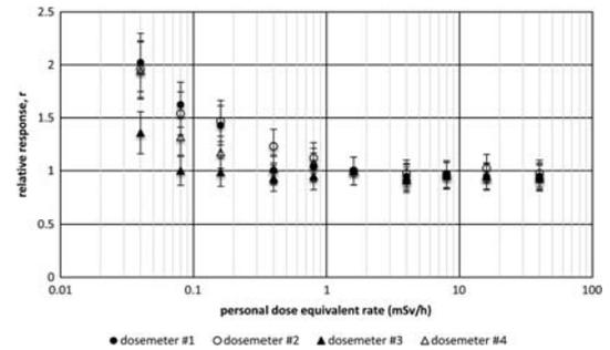
Figure 1. Results on the dose rate linearity of the all set of dosimeters.
