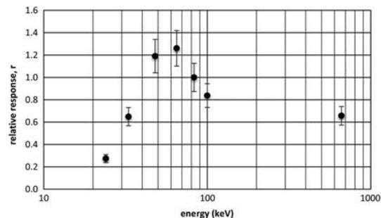
Figure 3. Results for energy dependence of the personal dosimeter.
