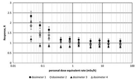
Figure 2. Response results of the overall dosimeters.
