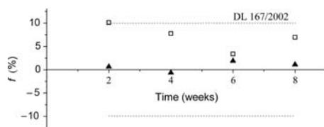
Figure 4. Fading effect for storage periods of 2, 4, 6 and 8 weeks for LiF:Mg,Ti (open squares) and LiF:Mg,Cu,P (closed triangles). The dashed lines represent an allowed variation of  $\pm 10\%$  per month<sup>(5)</sup>.
