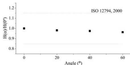
Figure 2. Angular dependence of the LiF:Mg,Ti dosimeter. The angles of incidence correspond to  $0^\circ$ ,  $\pm 20^\circ$ ,  $\pm 40^\circ$  and  $\pm 60^\circ$ .
