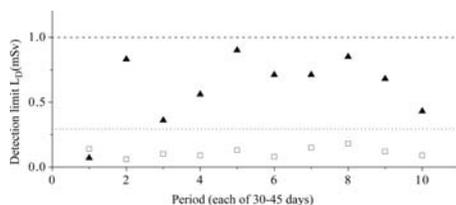
Figure 1. Calculation of the detection limit performed in 10 periods of 45 d: TLD-100H (closed triangles) and TLD-100 (open squares). The dotted line (at 0.3 mSv) and the dashed line (at 1 mSv) represent upper bounds for each set of data.
