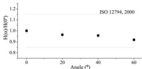
Figure 3. Angular dependence of the LiF:Mg,Cu,P dosimeter. The angles of incidence correspond to  $0^\circ$ ,  $\pm 20^\circ$ ,  $\pm 40^\circ$  and  $\pm 60^\circ$ .
