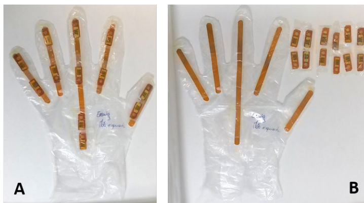
FIG. 1. The GafTLD glove used in P7 (see Fig. 5), with both TLDs and Gafchromic strips in place (a) and after removal of the TLDs (b); the darkening of the Gafchromic strips due to irradiation is visible. Order of fingers from left to right: little finger, ring finger, middle finger, index, and thumb (gloves worn on the left hand).
