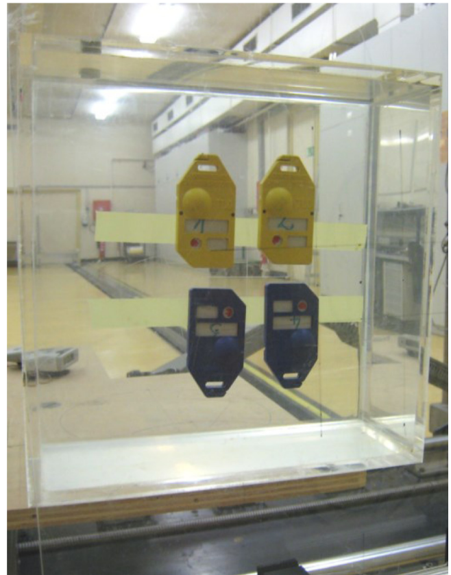
Fig. 1. Four whole-body dosimeters positioned on the front surface of the ISO water slab phantom.
