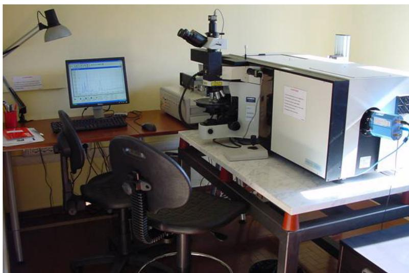
**Figure 19.** The μ-Raman Spectroscopy instrument
