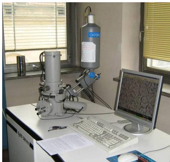
**Figure 14.** The SEM-EDX instrument
