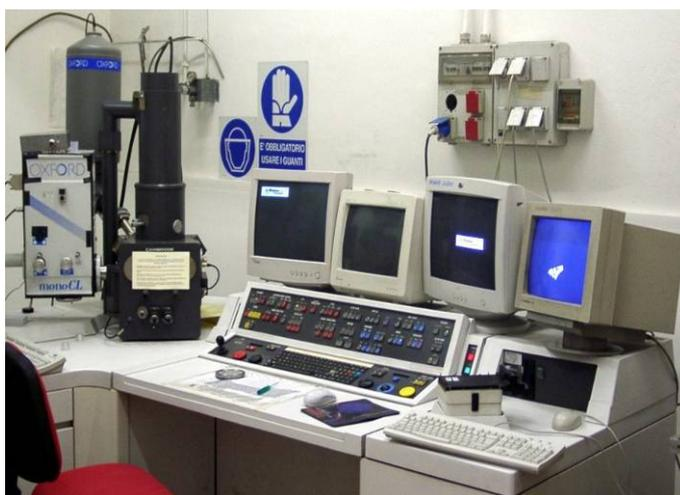
**Figure 15.** The SEM-CL instrument
