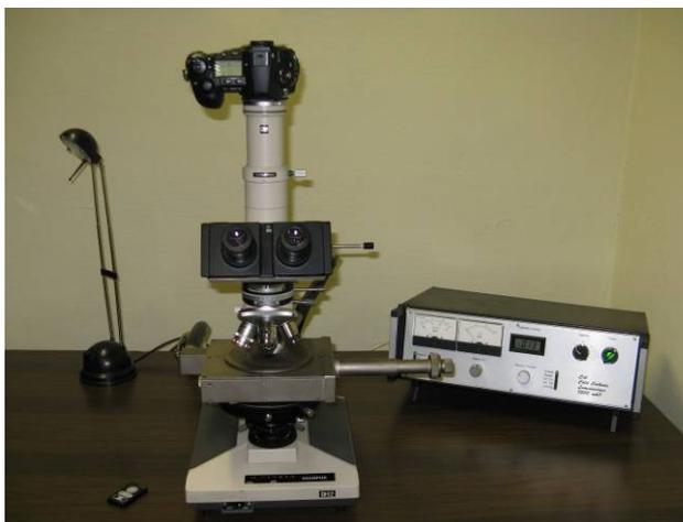
**Figure 13.** The cold-cathodoluminescence instrument
