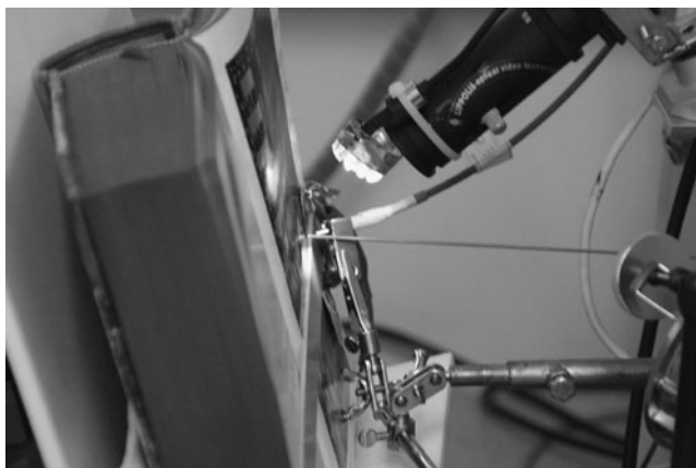
Fig. 3 AP/MALDI MS apparatus used for the direct spatially resolved study of printed books
