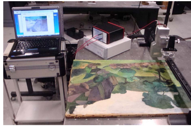
Fig. 1 Analysis of a painting with a compact portable LIBS spectrometer. (A probe head unit, containing a small nanosecond Nd:YAG laser, is positioned, with the aid of a micropositioning stage, over the painting. The LIBS emission signal is collected through the optical head and by optical fibers transmitted to a compact grating spectrograph equipped with a gated CCD detector controlled through a laptop computer [175])
