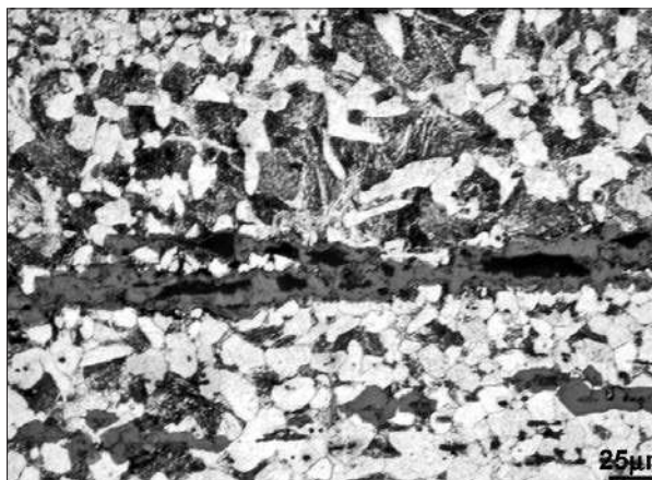
Fig. 17. - MOREIRINHA (PORTUGAL): metallography of the knife; detail of the union of the two piled sheets; some diffusion of carbon from the upper sheet to the lower one has occurred (etched with Nital).
