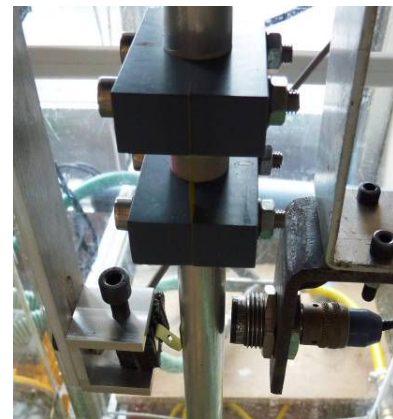
Figure 4. Electromagnetic lifting device (left) and eddy-current Kaman displacement transducer (right)
