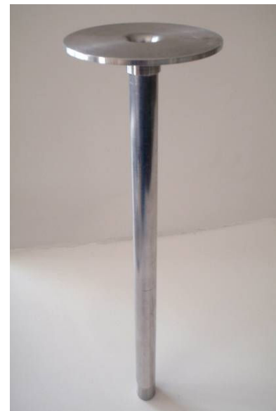
Figure 5. Baffled pipe with a smooth rounded water inlet, for a low value of the singular pressure loss
