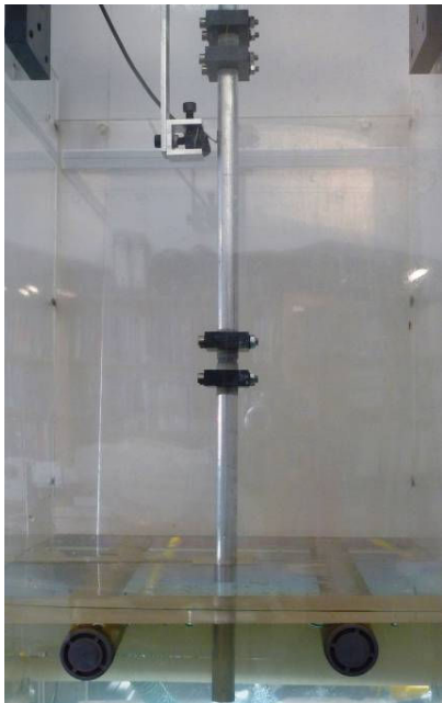
Figure 2. Experimental configuration with two articulated pipes
