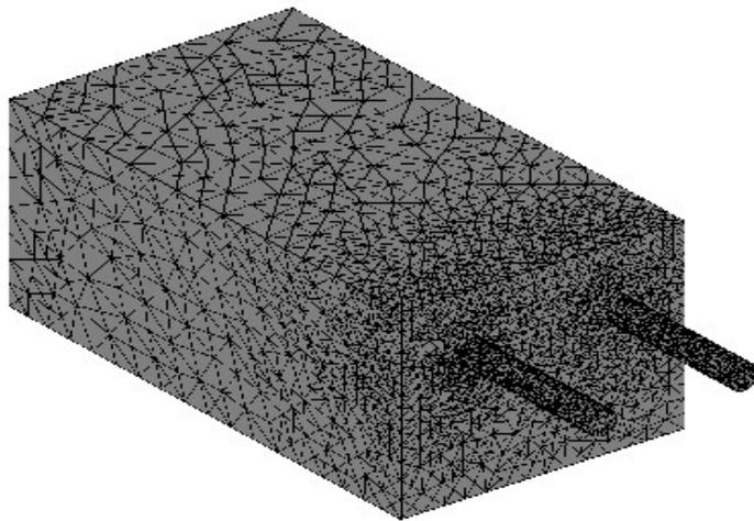
$$\begin{cases} L_x = 5 \text{ m}, L_y = 9 \text{ m}, L_z = 4 \text{ m} \\ L = 3 \text{ \& } 4.5 \text{ m}, D = 0.5 \text{ \& } 1 \text{ m} \end{cases}$$
