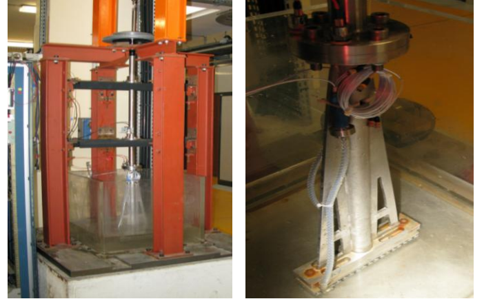
Figure 3: General view of the experimental rig and detail of the rigid instrumented plate.
