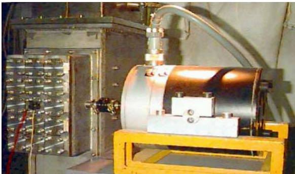
Figure 3: Electromagnetic shaker for feedback control of the tube damping and stabilization
