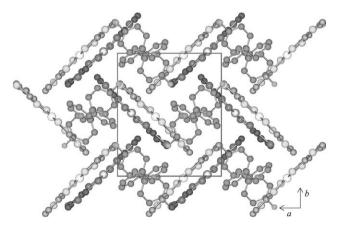
**Fig. 7** Crystal structure of **3** viewed along *c*: chains in adjacent layers alternating in dark and light grey.
