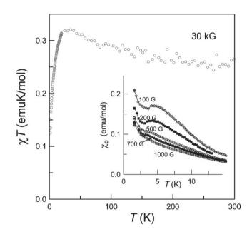
Fig. 13 Temperature dependence of  $\chi T$  for compound 2. The inset shows the paramagnetic susceptibility behaviour for various applied fields.
