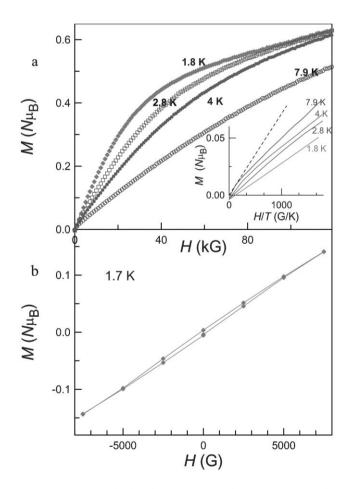
Fig. 14 (a) Magnetisation isotherms at various temperatures for compound 2. The inset shows the magnetisation at different temperatures as a function of H/T, the dashed line being the Brillouin function. (b) Magnetisation cycle at 1.7 K.
