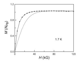
**Fig. 18** Magnetisation isothermal of compound **3**, at 1.7 K. The dashed line represents the calculated values from the Brillouin function.
