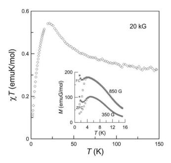
**Fig. 9** Temperature dependence of  $\chi T$  for compound 1, under an applied field of 20 kG. The inset shows the ZFC (open symbols) and FC (closed symbols) magnetization curves for applied fields of 350 and 850 G, represented by circles and squares respectively.
