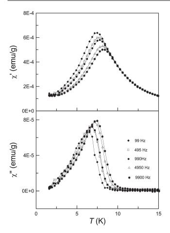
Fig. 11 (a) Real component of AC susceptibility,  $\chi'$ , temperature dependence for compound 1. (b) Imaginary component,  $\chi''$ , temperature dependence.
