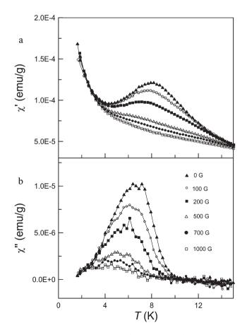
Fig. 15 Temperature dependence of real,  $\chi'$ , (a) and imaginary,  $\chi''$ , (b) components of AC susceptibility of compound 2 under different indicated values of applied DC field.
