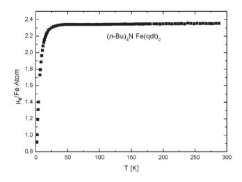
Fig. 4 Effective magnetic moment,  $\mu_{\rm B}$ , of 1 as a function of temperature, *T*.
