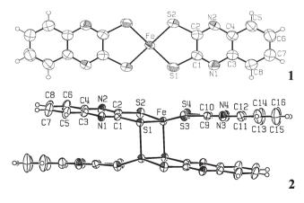
Fig. 1 ORTEP diagrams of the  $Fe(qdt)_2^-$  complexes in 1 and 2. Fe–S bond lengths in 1 are 2.1729(14) Å and 2.1770(14) Å, shorter than the corresponding basal Fe–S distances in 2, 2.2259(13), 2.2289(13), 2.2436(13) and 2.2368(12) Å. The apical distance is 2.4884(13) Å. Displacement ellipsoids are drawn at the 40% probability level and H atoms are shown as small spheres of arbitrary radii.
