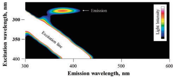
**Fig. 1.** Excitation (vertical axis) and emission (horizontal axis) map of  $\text{Ga}_2\text{O}_3$ .
