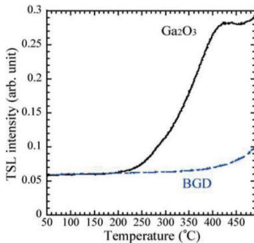
**Fig. 6.** TSL glow curve of  $\text{Ga}_2\text{O}_3$  after irradiation with X-rays with a dose of 1 Gy. The background (BGD) signal measured without the sample is superposed.
