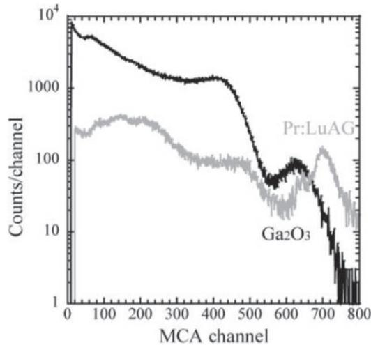
**Fig. 5.**  $^{137}\text{Cs}$   $\gamma$ -ray-irradiated pulse height spectrum of  $\text{Ga}_2\text{O}_3$  and Pr-doped LuAG.
