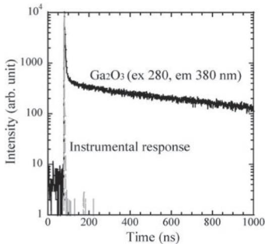
**Fig. 2.** PL decay time profile of  $\text{Ga}_2\text{O}_3$  monitoring at a wavelength of 380 nm under an excitation wavelength of 280 nm.
