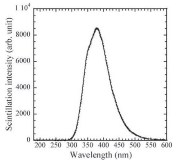
**Fig. 3.** X-ray-induced scintillation spectrum of  $\text{Ga}_2\text{O}_3$ .
