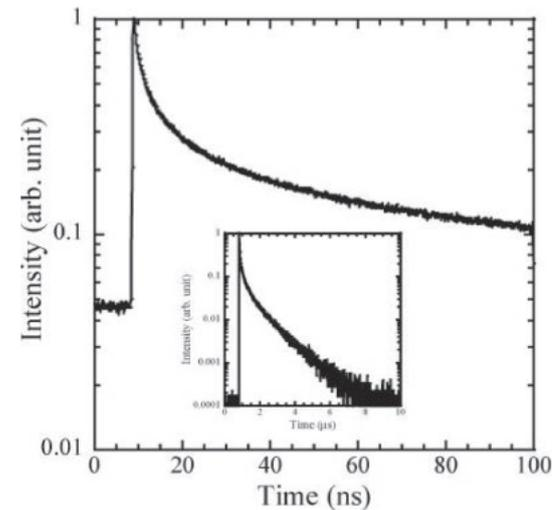
**Fig. 4.** X-ray-induced scintillation decay time profile of  $\text{Ga}_2\text{O}_3$ . The inset expands the time range to 10  $\mu\text{s}$  to show the slower component.
