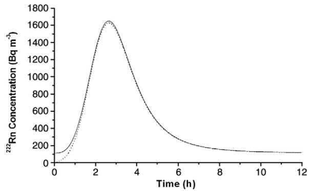
Fig. 6. Characteristic case of modelling of radon concentration ( $A_0$ ) in a TR of the BMTS of the Loutraki spas ( $i/i=7$ , Fig. 5). The dotted curve refers to the fitted time-series  $A_0$  functions of AG. The other curve refers to the modelled  $A_0$  data.
