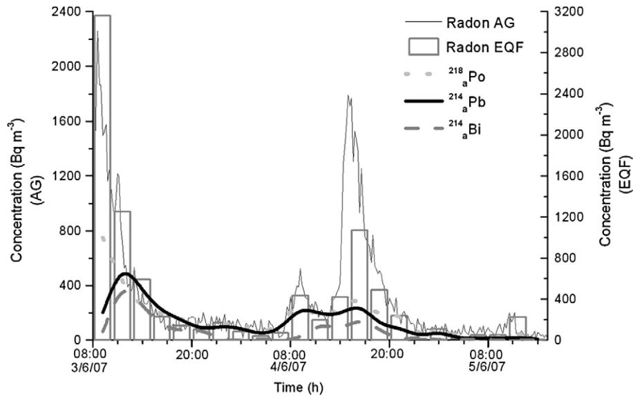
Fig. 2. First characteristic case of radon and progeny transient activity concentration variations recorded by AG and EQF in the ambient air of a TR of the BMTS. Only the attached progeny concentrations are presented for convenience.
