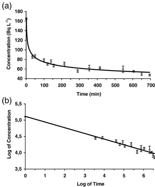
Fig. 4. (a) Measurements of the time variations of the radon concentrations of the bathtub spring water, (b) Fitted power model curve of Eq. (1.2) linearly transformed.
