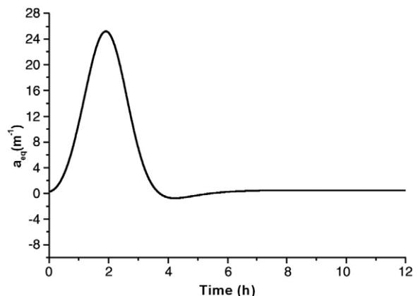
Fig. 7. Variations of the specific total interfacial area ( $a_{eq}$ ) of Fig. 6 obtained from the modelling according to Eqs. (1.1) and (1.2).
