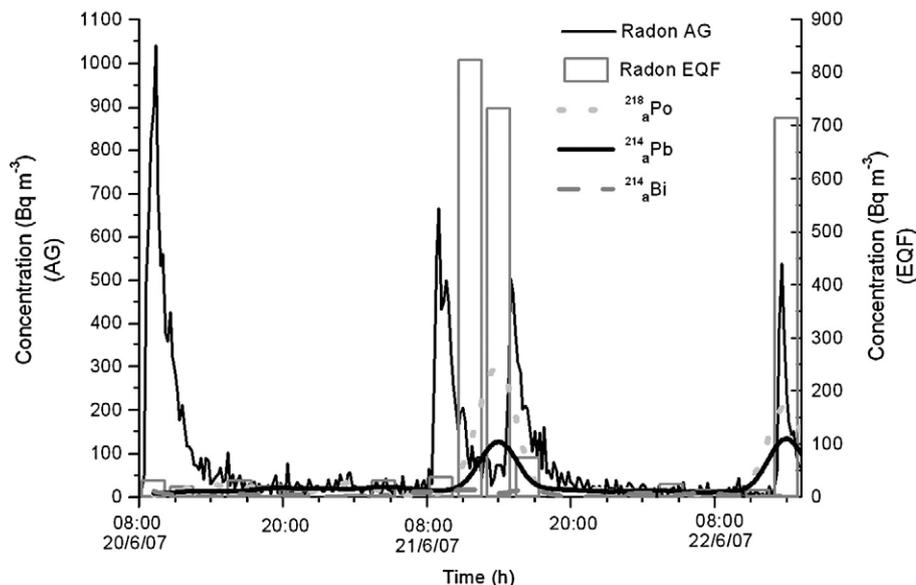
Fig. 3. Second characteristic case of radon and progeny transient activity concentration variations recorded by AG and EQF in the ambient air of a TR of the BMTS. Only the attached progeny concentrations are presented for convenience.
