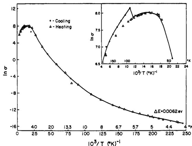
Figure 1. Natural logarithm of  $\sigma$  in  $\text{ohm}^{-1} \text{cm}^{-1}$  vs.  $10^3/T$  for sample no. JPF-5.  $\Delta E$  is calculated from  $\sigma = \sigma_0 e^{-\Delta E/2kT}$ . Insert shows high-temperature region expanded showing hysteresis between cooling and heating curves at the transition; cooling curve determined first.
