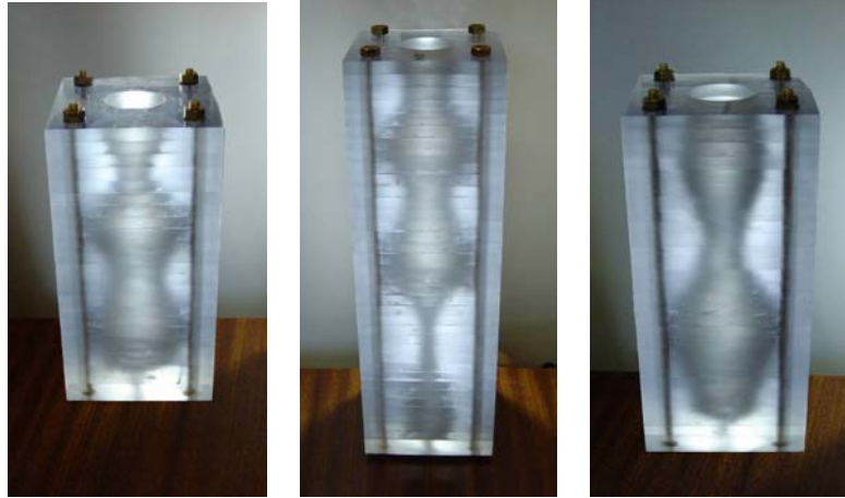
Figure 6 – Optimized resonators. From left to right: 1:4:10; 1:1.67:4:10 and 1:4:6.67:10.
