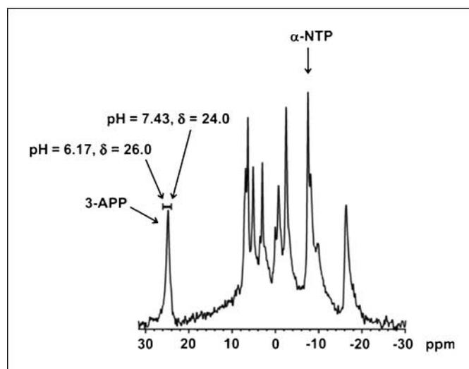
**Figure 4.** *In vivo*  $^{31}\text{P}$  MRS of a PC-3 tumor.  $\text{pH}_e$  is estimated from the chemical shift difference (in ppm) between the  $\text{pH}_e$  indicator 3-APP and the pH-independent chemical shift of  $\alpha$ -nucleoside triphosphate ( $\alpha$ -NTP). The scale bar above the 3-APP resonance indicates a range of chemical shifts ( $\delta$ ) from 24.0 to 26.0 ppm, corresponding to the physiologic range of  $\text{pH}_e$  (6.17-7.43).
