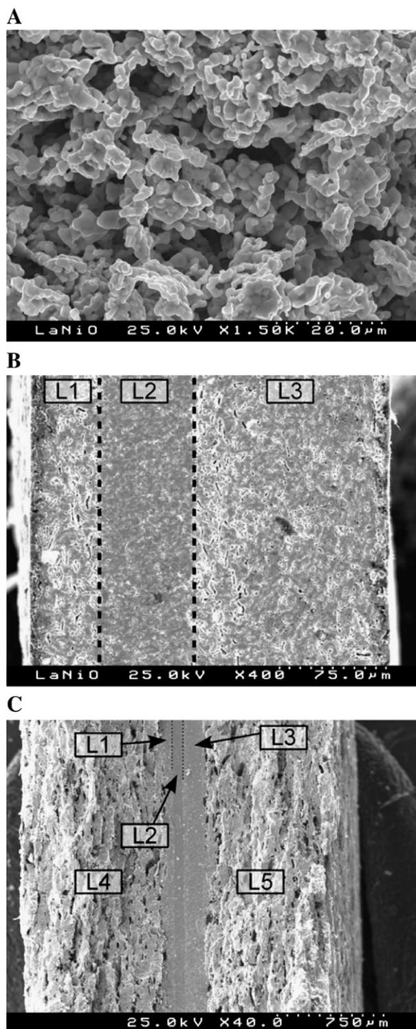
Fig. 1. SEM micrographs of the activated feed-side surface of monolayer  $\text{La}_2\text{NiO}_{4+\delta}$  membrane (A), and cross-sections of 3-layer (B) and 5-layer (C) ceramics. For (B) and (C), L2 corresponds to the dense central layer; L1 and L3 are thin porous layers. L4 and L5 in (C) correspond to the additional porous layers.
