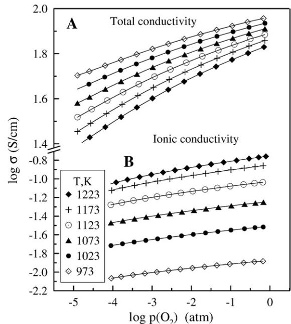
Fig. 4. Oxygen partial pressure dependencies of the total (A) and oxygen ionic (B) conductivities of  $\text{La}_2\text{NiO}_{4+\delta}$ . The ionic conductivity was calculated numerically from the oxygen permeation, nonstoichiometry and total conductivity data using Model 1 (see text).
