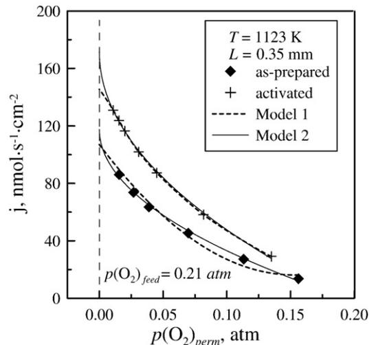
**Fig. 7.** Comparison of the fitting results using Models 1 and 2, for the tape-casted 1-layer membranes with and without surface modification.
