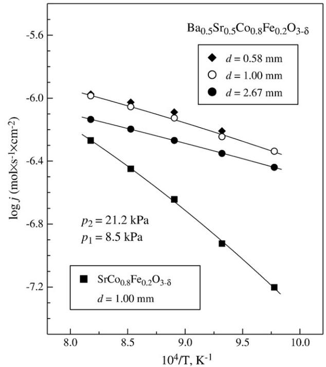
**Fig. 3.** Oxygen permeation fluxes through dense BSCF membranes with different thicknesses under a fixed  $p(\text{O}_2)$  gradient. Data on SrCo<sub>0.8</sub>Fe<sub>0.2</sub>O<sub>3-δ</sub> [17] are shown for comparison. All data correspond to membranes without surface modification; the measurements were performed by Method 1.
