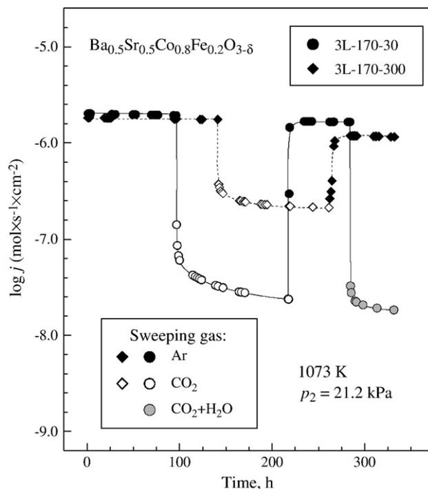
**Fig. 5.** Time dependence of oxygen permeation fluxes through three-layer BSCF membranes exposed to CO<sub>2</sub>- and H<sub>2</sub>O-containing atmospheres. Sweeping gas flow rate: 25 cm<sup>3</sup>/min; p(O<sub>2</sub>) in inlet Ar flow: ~10 Pa, p(O<sub>2</sub>) in inlet CO<sub>2</sub> flow: ~5 Pa, p(H<sub>2</sub>O) in inlet (CO<sub>2</sub> + H<sub>2</sub>O) flow: ~2.6 kPa.
