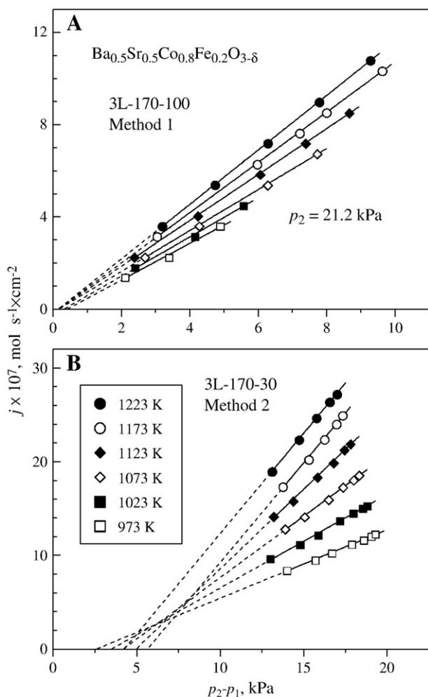
**Fig. 4.** Dependence of oxygen permeation fluxes through three-layer BSCF membranes on oxygen partial pressure difference at various temperatures. The measurements were performed by Method 1 (A) without supplying gas flow to the membrane surface, and by Method 2 (B) when the permeate-side surface was exposed to Ar–O<sub>2</sub> flow.
