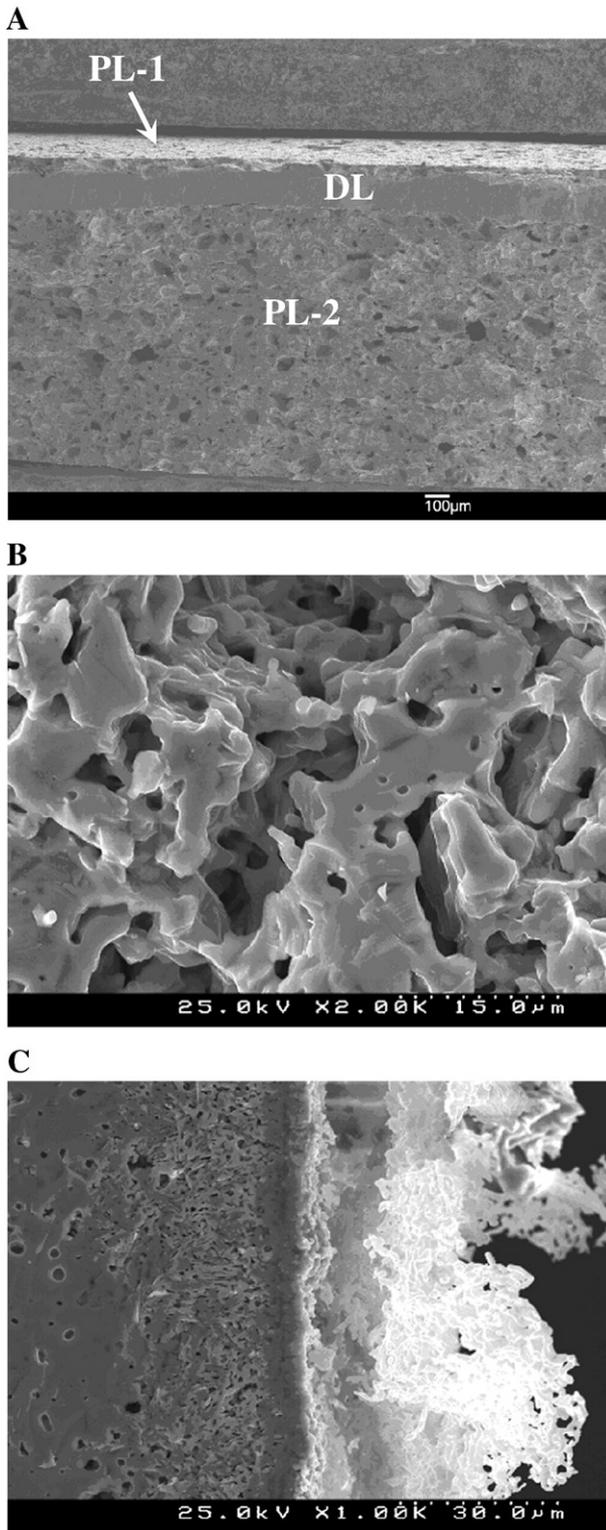
**Fig. 2.** SEM micrographs of a three-layer 3L-170-60 membrane after fabrication (A) and after testing in CO<sub>2</sub>: surface of the feed-side porous layer (B) and cross-section near the permeate side exposed to CO<sub>2</sub> (C). The abbreviations PL-1, DL and PL-2 on micrograph (A) denote thin porous, dense and thick porous support layers, correspondingly. The micrograph (C) shows the dense BSCF layer (left), porous permeate-side layer (center), and carbonate containing layer.
