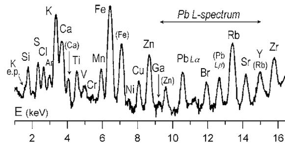
**FIGURE 2** SRXRF spectrum (excitation energy 18.9 keV) collected from an encrustation of *Xanthoria parietina* lichen over a granite stone
