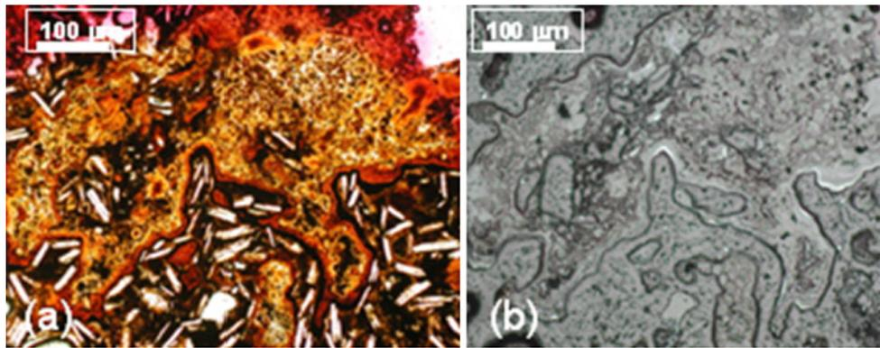
**Fig. 4** Photo-micrographs illustrating the late Fe<sup>3+</sup>-bearing precipitates in AM-V sample (AC1 drill-hole). Transmitted, simply polarised light for image **a**; reflected, simply polarised light for **b** image,
