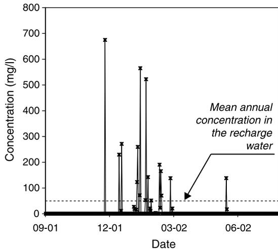
Fig. 5. Variations of nitrate concentration in the groundwater recharge (crosses) calculated from the nitrogen excess in 2000–2001. The mean annual nitrate concentration is also represented (dashed line).
