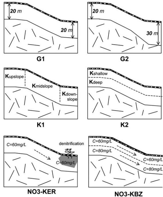
Fig. 4. Sketch diagrams of the flow-model geometries (G1 and G2), the spatial distribution of hydraulic conductivity (K1 and K2) and the spatial distribution of nitrate concentrations in the groundwater (NO3-KER and NO3-KBZ). Values of hydraulic conductivities are specified in Table 2.
