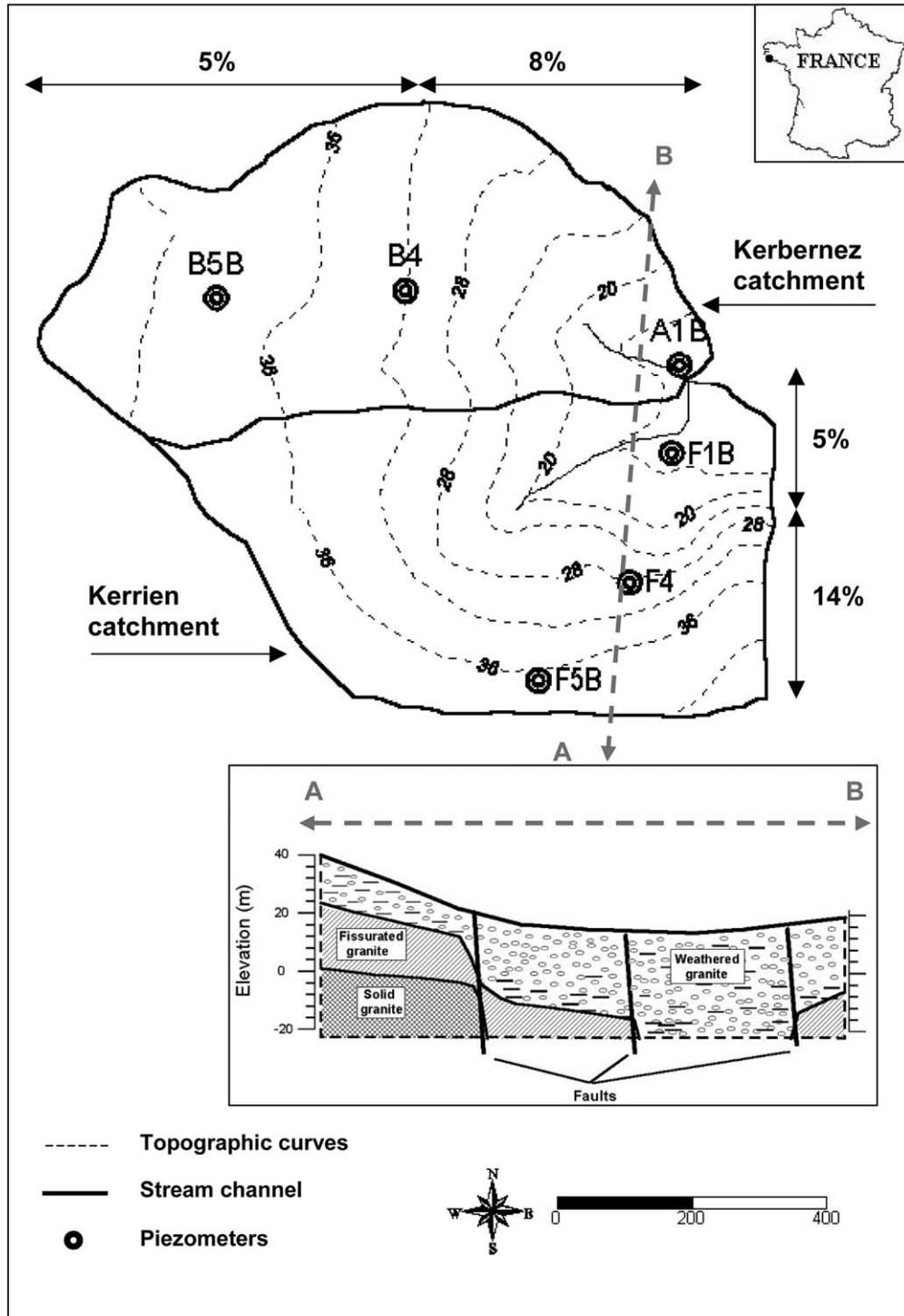
Fig. 1. Study site location: piezometer positions, surface slopes and geological cross-section along the AB profile, inferred from geophysical measurements in the Kerbernez and Kerrien catchments (adapted from Legchenko et al. (2004)).
