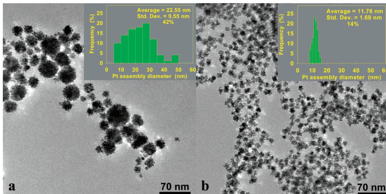
**Figure 4.** TEM images of platinum nanostructures produced in the presence of SDS without (a) and with (b) photocatalyst and their respective size distributions (insets). Average diameters were measured for 100 nanostructures, and their frequencies are plotted in the inset graphs. The average size and the standard deviations are given in the plots, along with the percentage ratio of the standard deviation to average size.
