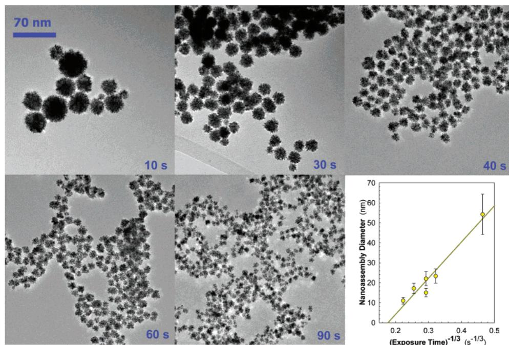
**Figure 7.** TEM images of the nanostructures as a function of intense light exposure time and the relationship between the average diameter of the nanostructures and the cube root of the inverse of the exposure time.
