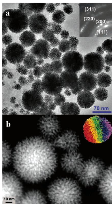
**Figure 3.** (a) TEM image of nanodendrites produced with Brij-35 surfactant in the absence of photocatalyst and (inset) the electron diffraction pattern of a group of the dendrites indicating that they are composed of platinum metal and as a group are polycrystalline. (b) HAADF scanning TEM image of the three-dimensional platinum dendrites grown in the presence of Brij-35 micelles. Inset: a Koosh ball.
