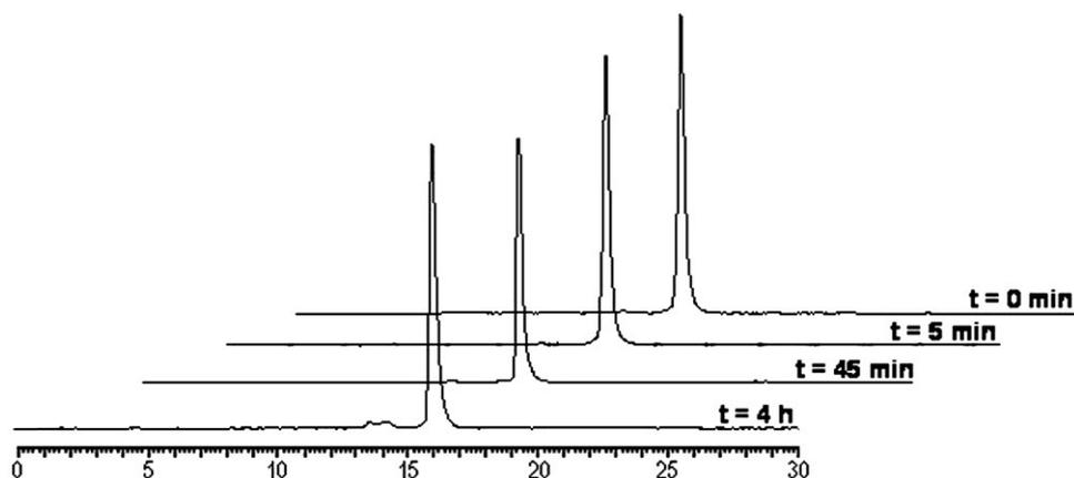
Fig. 3. RP-HPLC profile of  $[\text{Ac-Nle}^4, \text{Asp}^5, \text{D-Phe}^7, \text{Lys}^{11}(\text{pz-}^{99\text{m}}\text{Tc}(\text{CO})_3)]\alpha\text{-MSH}_{4-11}$  ( $t_r=16.0$  min) after incubation in fresh human plasma at different time points.
