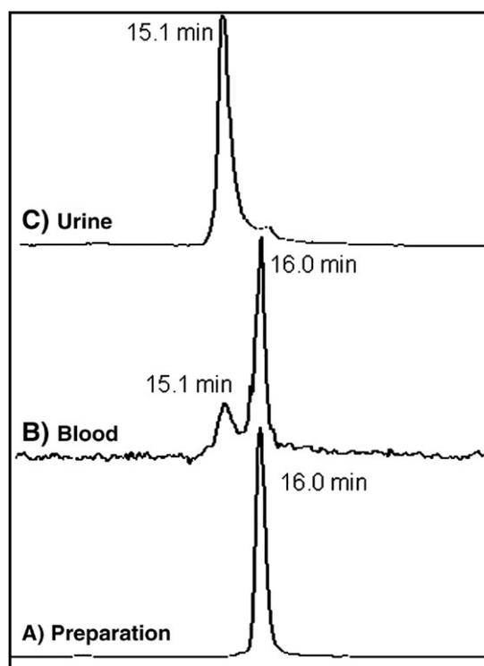
Fig. 6. RP-HPLC chromatograms of the injected preparation (A), blood serum (B) and urine (C) samples collected at 1 h p.i.
