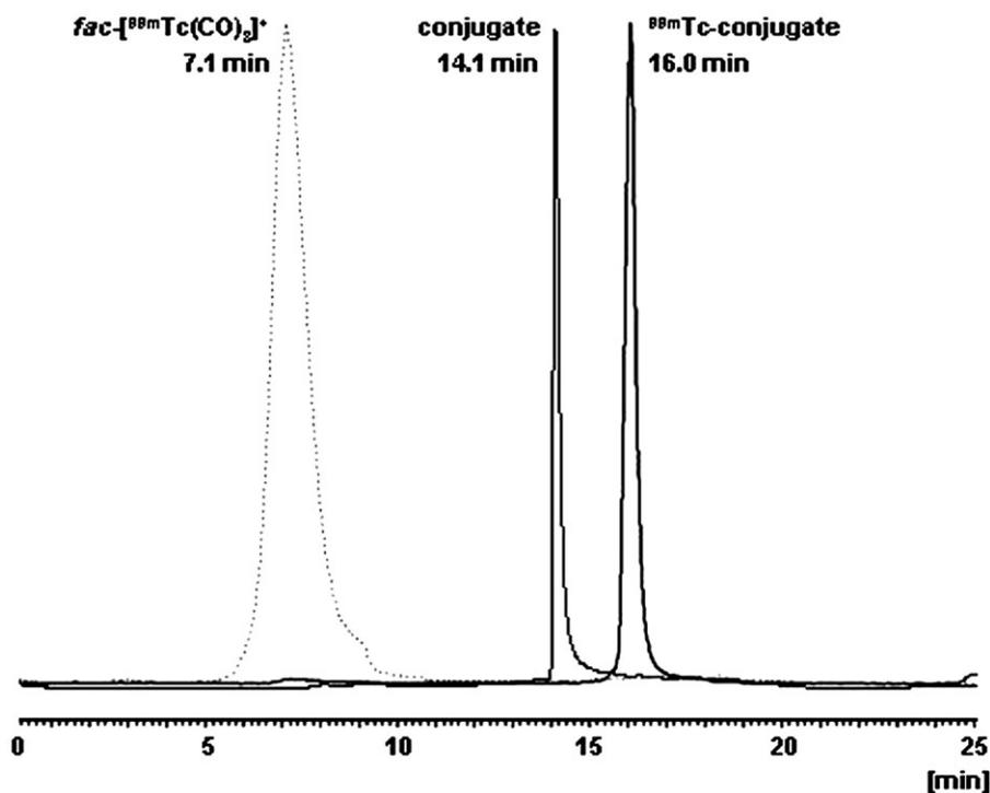
Fig. 2. Superimposition of RP-HPLC chromatograms of the precursor *fac*-[<sup>99m</sup>Tc(CO)<sub>3</sub>(H<sub>2</sub>O)<sub>3</sub>], [Ac-Nle<sup>4</sup>,Asp<sup>5</sup>,D-Phe<sup>7</sup>,Lys<sup>11</sup>(pz-<sup>99m</sup>Tc(CO)<sub>3</sub>)]α-MSH<sub>4–11</sub> (γ detection) and the peptide conjugate [Ac-Nle<sup>4</sup>,Asp<sup>5</sup>,D-Phe<sup>7</sup>,Lys<sup>11</sup>(pz)]α-MSH<sub>4–11</sub> (UV detection, 280 nm).
