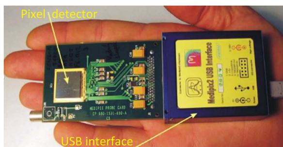
Fig. 3. Developed NORM Pixel detector with USB interface.
