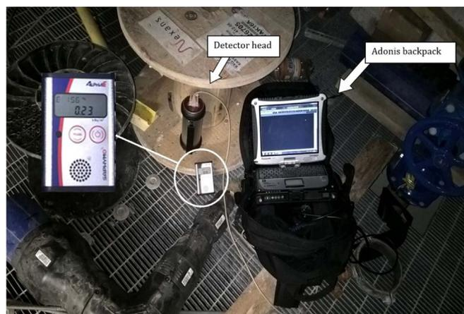
Fig. 1. The MetroNORM in-situ alpha-spectrometer system Adonis in operation.
