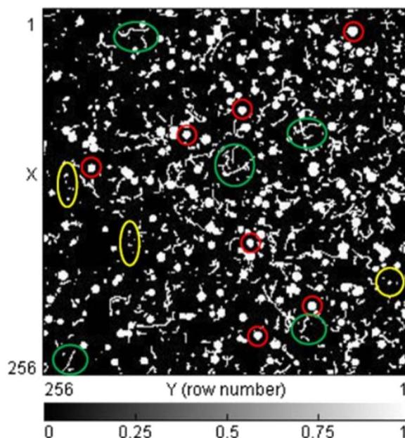
Fig. 4. NORM Alpha-particle (red, small circles), beta-particle (green, bigger circles) and gamma-ray (yellow, ovals) response at the pixel detector. (For interpretation of the references to color in this figure legend, the reader is referred to the web version of this article).
