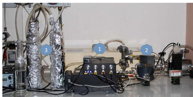
Fig. 5.  $^{220}\text{Rn}$  measurement setup with  $^{228}\text{Th}$  source (1),  $^{220}\text{Rn}$  chamber (2) and gas bubblers with liquid scintillator (3).
