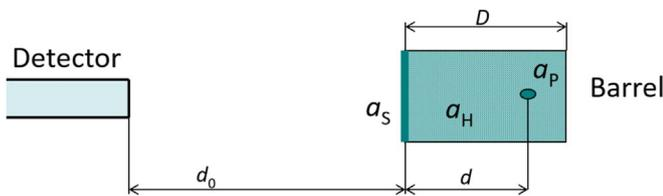
Fig. 6. Detection of inhomogeneity in NORM waste drums: Three distinct contributions to radioactivity distribution supposed: surface ( $a_S$ ), homogeneous ( $a_H$ ) and point source ( $a_P$ ) contributions.
