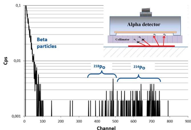
Fig. 2. Spectrum of  $^{222}\text{Rn}$  progenies at the testing operation of the in-situ alpha spectrometer Adonis with collimator.
