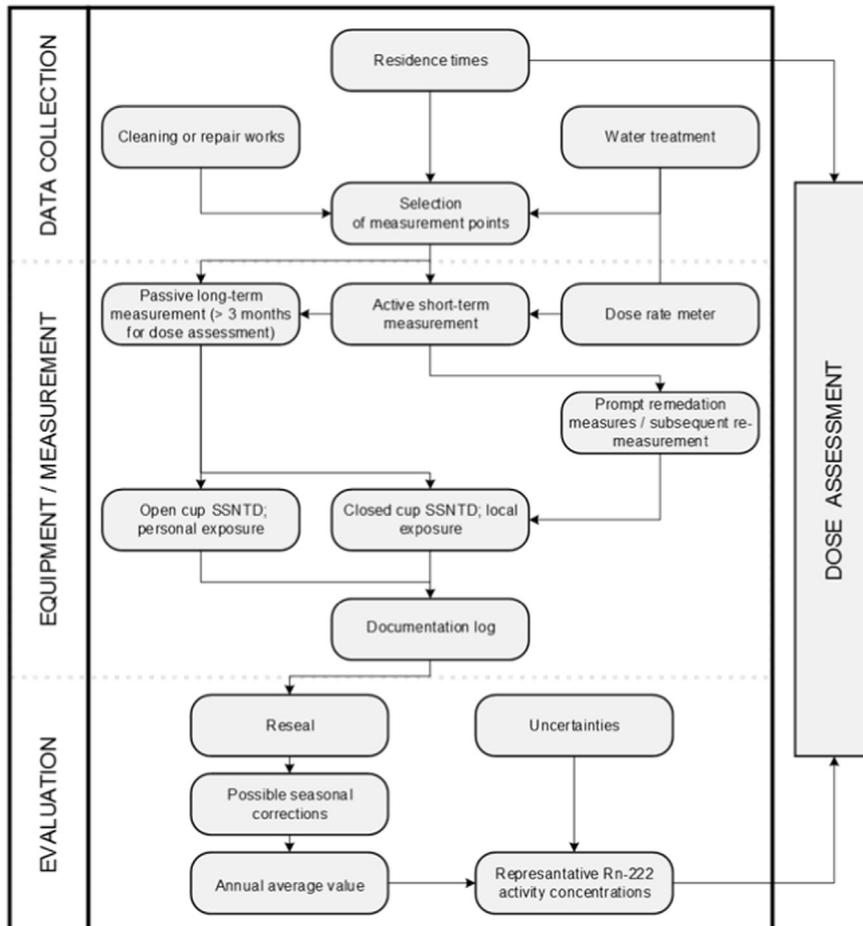
Fig. 7. Scheme of the in-situ method for exposure and dose assessment of radon in drinking water plants.
