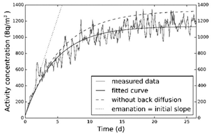
Fig. 8. Radon emanation measurement of building materials.
