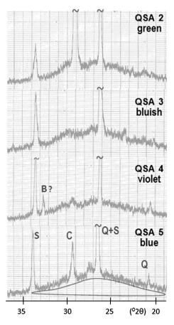
**Fig. 3.** XRD patterns collected from 18th century glaze fragments (QSA – *Quinta de Santo António*). The contribution of an amorphous phase is assigned; identified crystalline phases: S, cassiterite (SnO<sub>2</sub>); Q, quartz (SiO<sub>2</sub>); C, calcite (CaCO<sub>3</sub>); B?, braunite (3Mn<sub>2</sub>O<sub>3</sub>·MnSiO<sub>3</sub>).
