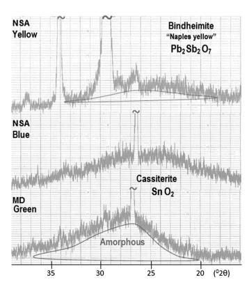
**Fig. 2.** X-ray diffraction (XRD) patterns (Cu  $K\alpha$  radiation) collected from glaze fragments: MD – *Madre de Deus* Church (16th century); NSA – *Nossa Senhora dos Aflitos* Church (17th century).
