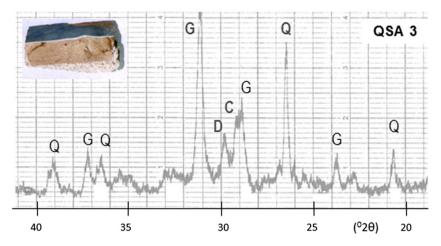
Fig. 4. XRD pattern collected from the ceramic body of a QSA tile sample. Assigned phases by decreasing representativity: G, gehlenite (CaAl<sub>2</sub>SiO<sub>7</sub>); Q, quartz (SiO<sub>2</sub>); D, diopside (CaMgSi<sub>2</sub>O<sub>6</sub>); C, calcite (CaCO<sub>3</sub>).
