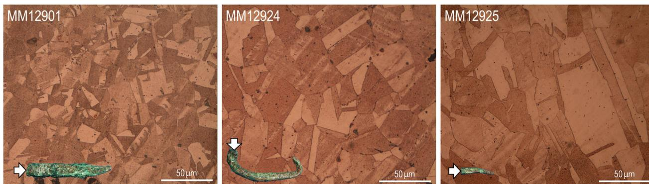
**Fig. 4** Microstructures of nails MM12901, MM12924 and MM12925 (bright field, etched; *bottom left* observed sections of nails, the *left* nail has 3.1 cm length, and the remaining are on the same scale)
