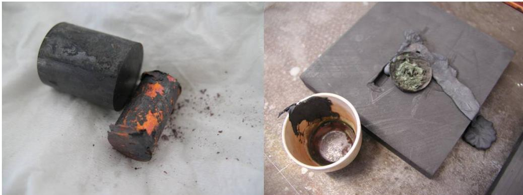
**Fig. 3.12** Laboratorial experiments showing the formation of a surface layer of tenorite. At left, the annealing of copper-based metal bars and at right the pouring of metal to an open mould.
