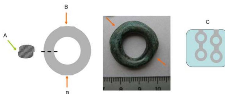
**Fig. 3.36** Casting defects resulting from a bivalve mould. At left a scheme with the casting defects observed on the ring MED-22: (A) inadequate matching among the two halves and (B) irregular surfaces after casting sprue. At the centre a photograph of MED-22, with the positioning of the (B) defects depicted. At the right (C) a scheme representing the interpretation of a possible bivalve mould for casting various rings.
