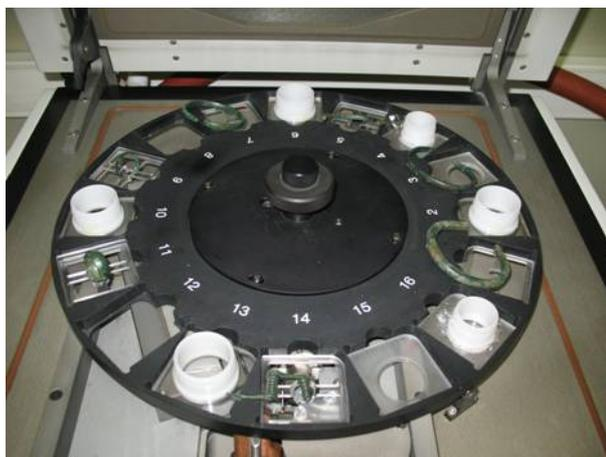
**Fig. 1.3** Kevex 771 chamber (EDXRF) with artefacts from *Medronhal* placed in the rotating 16-position sample tray.
