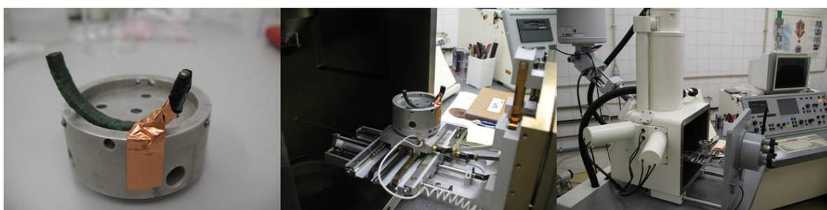
Fig. 1.7 Preparation of a bracelet fragment from *Medronhal* for SEM-EDS analysis and its placement in the Zeiss model DSM 962 equipment chamber.
