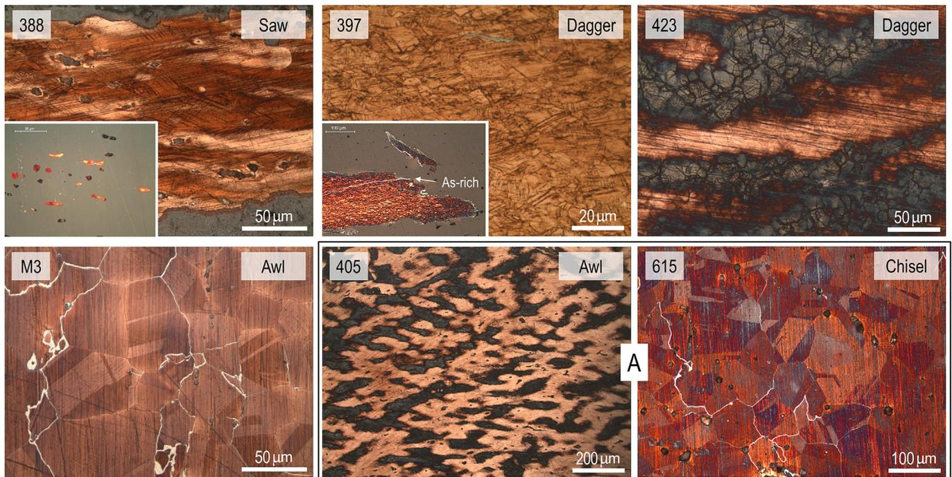
**Fig. 3.** Microstructures of MBA arsenical copper artefacts from Torre Velha 3 and Monte da Cabida 3 (A: unusual microstructures).
